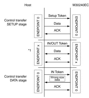
Case 3: At Control Read transfer DATA stage, M30240EC sends wrong size data.
