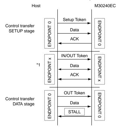
Case 1: At Control Write transfer DATA stage, M30240EC sends STALL for the handshake.
