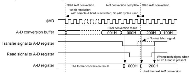
Normally, A-D conversion value is saved at the rising edge (dashed rising edge) of the latch signal. However, when the CPU is doing a read to A-D register at this time, the A-D register latch signal is delayed, and wrong value is stored at A-D conversion register.
