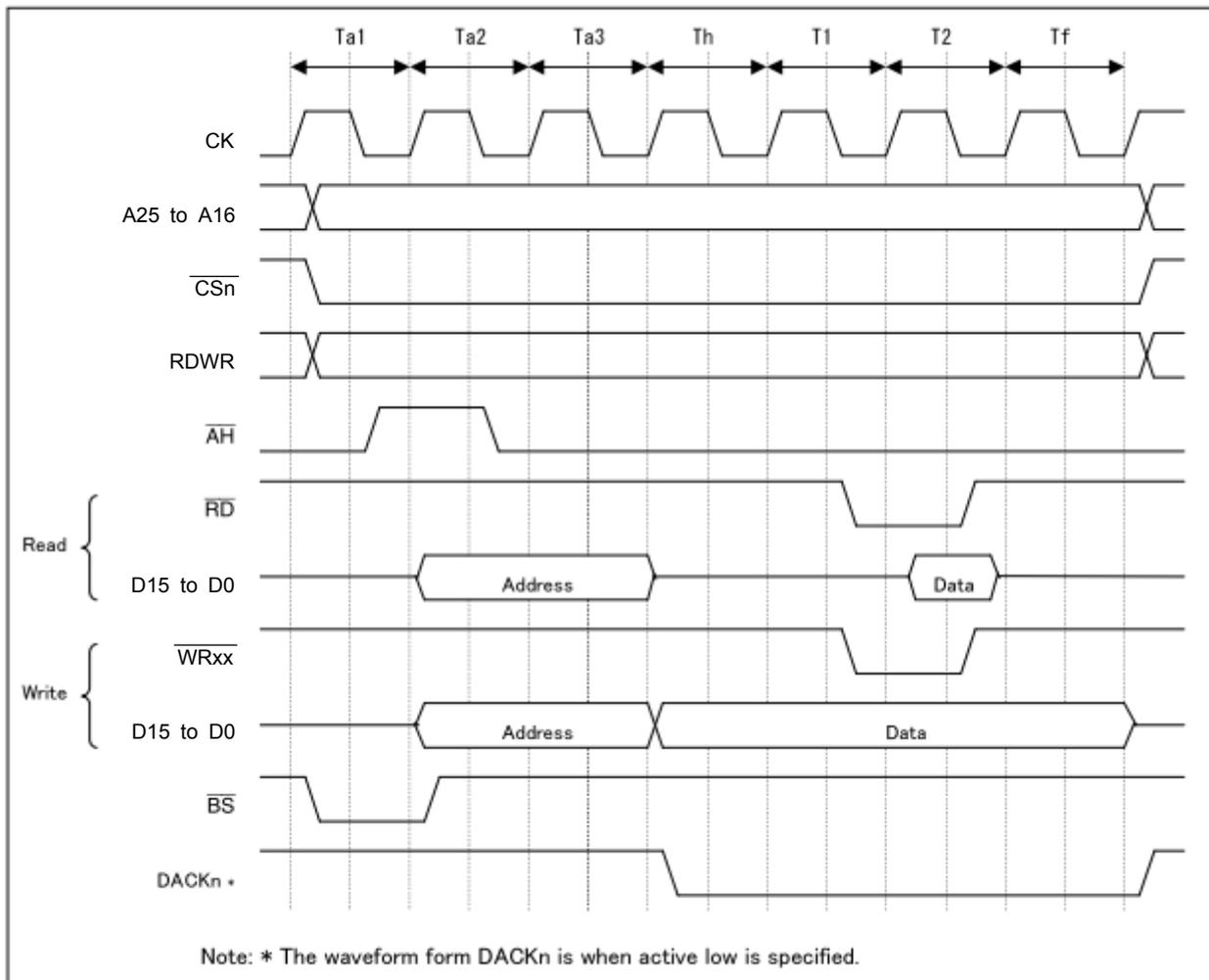
**Figure 9.11 (2) Access Timing for MPX Space**
