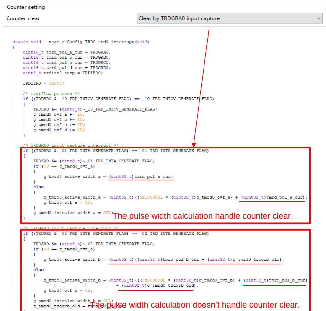
Figure 6-3 Counter clear setting in Input capture function
