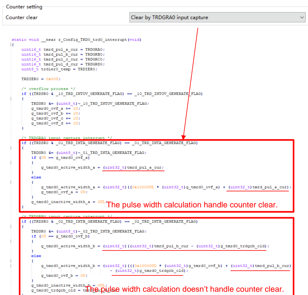
Figure 6-3 Counter clear setting in Input capture function
