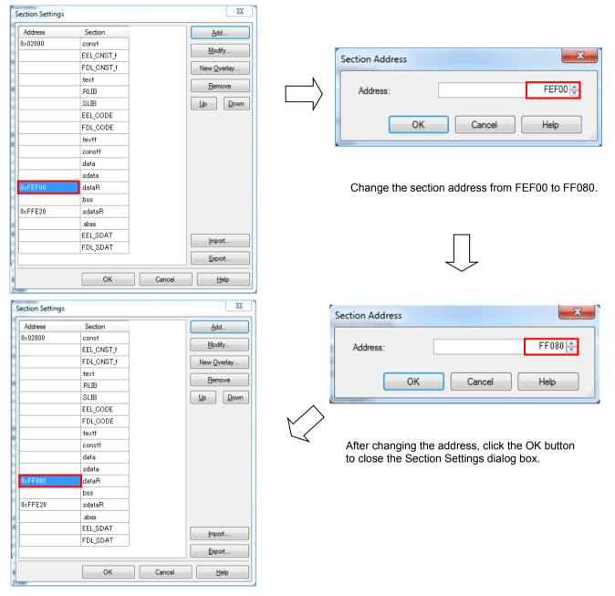
Figure 8-3. Example of Changing the User RAM Area Allocation (RAM Area)
