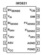
Figure 4.1 : 14-Lead SOIC-14 Package
