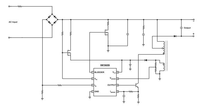
Figure 3.1 : iW3609 Simplified Application Circuit
