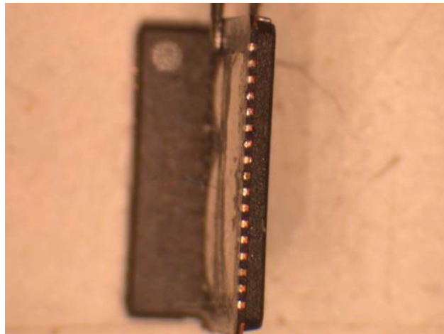
Figure 17. Finished Tinned Thermal Land on QFN
