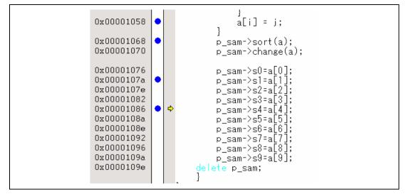
Figure 2.2 [Source] Window at Execution Halted (Sequential Break)
