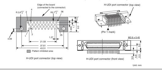
Figure 1.2 Pin Assignments of the H-UDI Port Connector (36 Pins)
