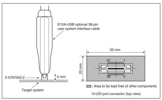
Figure 1.1 Restriction on Component Mounting
