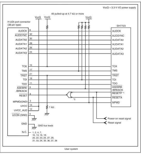
Figure 1.7 Recommended Circuit for Connection between the H-UDI Port Connector and MPU when the Emulator is in Use (38-Pin Type)
