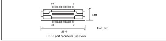
Figure 1.4 Pin Assignments of the H-UDI Port Connector (38 Pins)
