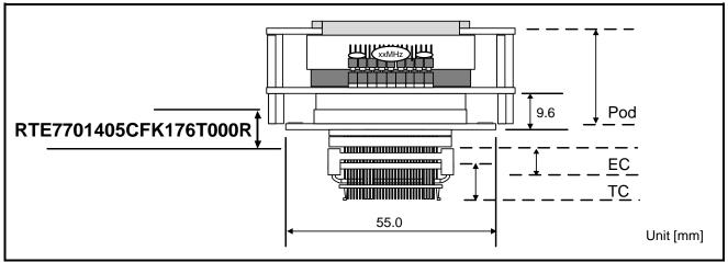
Figure 4 Drawing of the Socket Assembly
