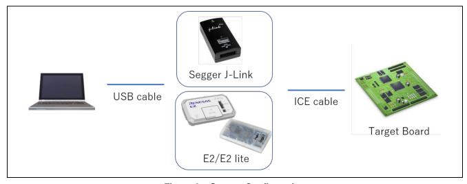
Figure 2. System Configuration
