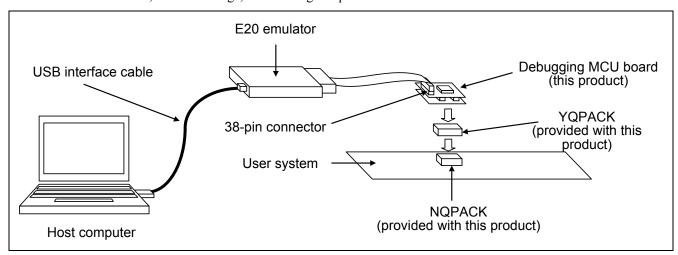
Figure 1 System Configuration
