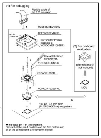
Figure 3 Connection of the User System and This
