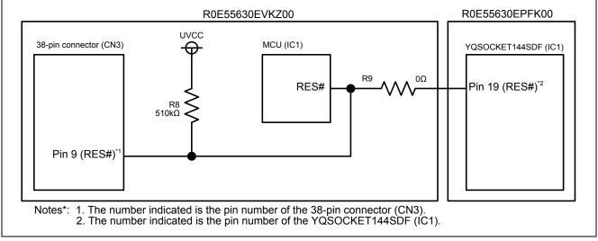
Figure 2 Reset Circuit on the Debugging MCU Board
