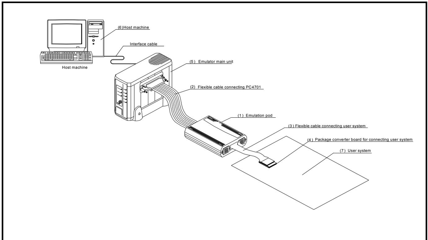
Figure 1.1 System configuration
