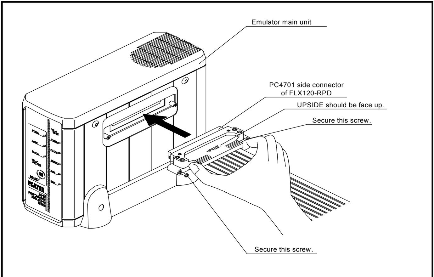
Figure 2.2 Connecting the FLX120-RPD to the PC4701
