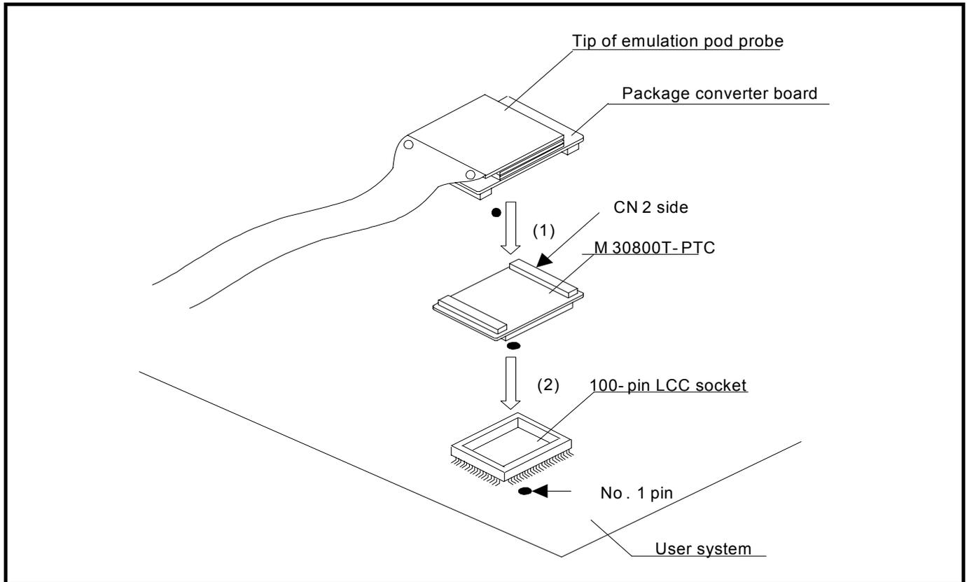
Figure 2.10 Connecting to a 100-pin LCC socket
