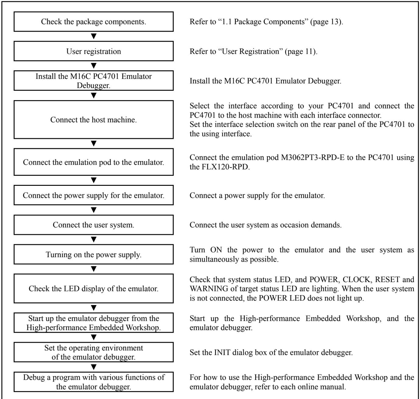
Figure 2.1 Flowchart of starting up the emulator
