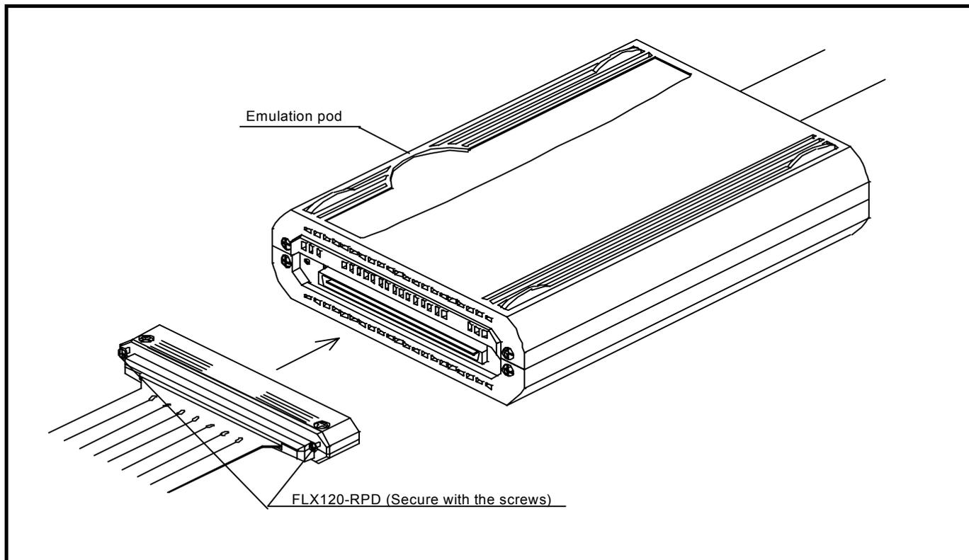
Figure 2.3 Connecting the FLX120-RPD to the emulation pod
