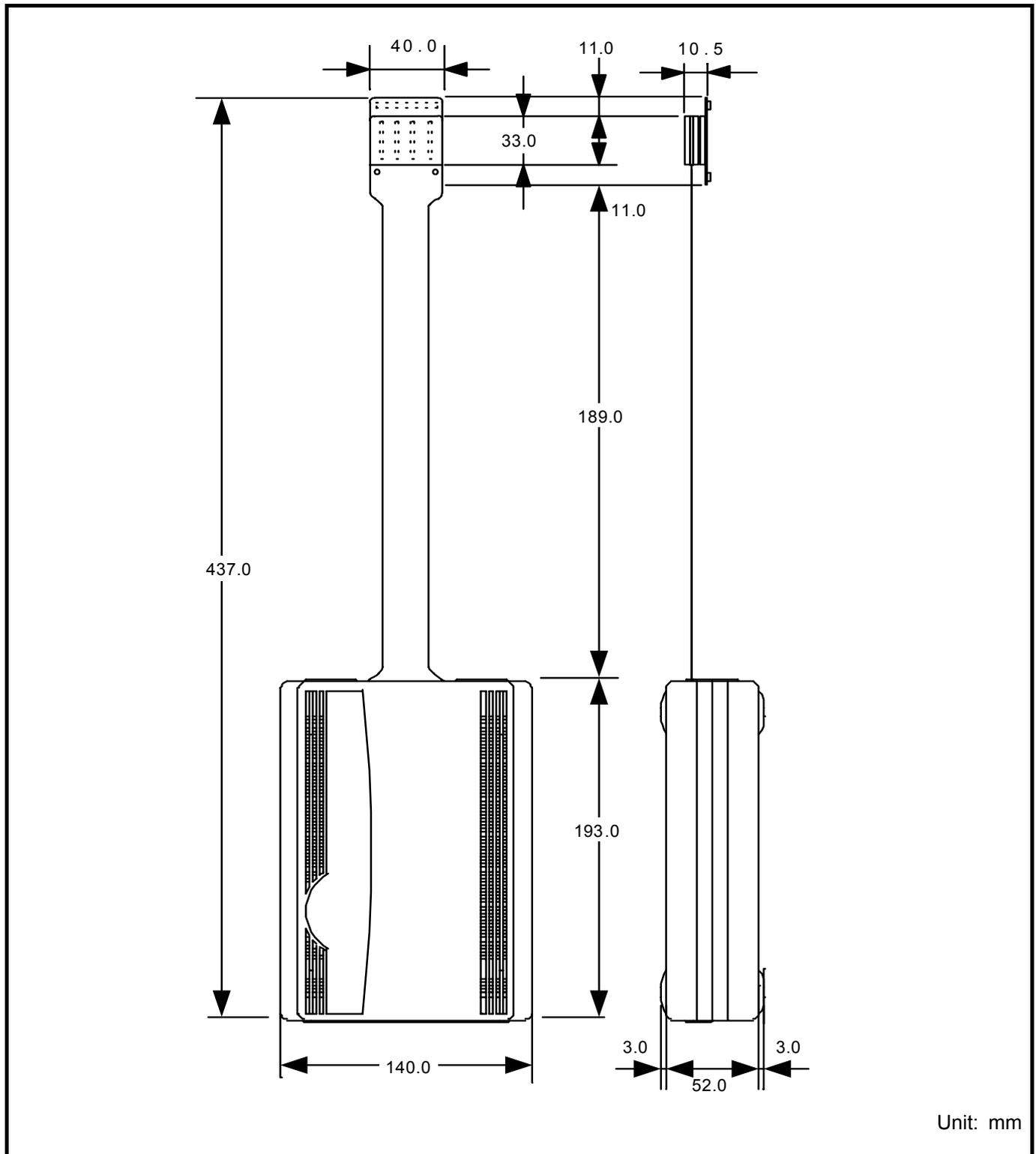
Figure 4.8 External dimensions of the emulation pod
