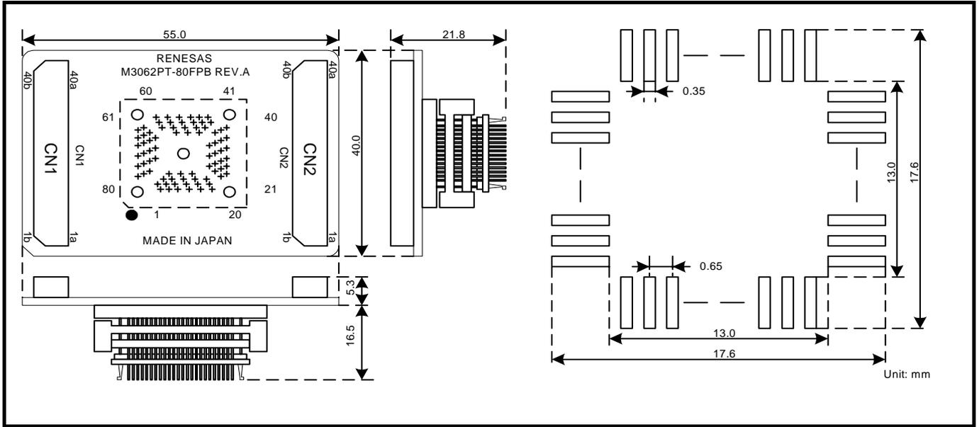
Figure 4.10 External dimensions and a sample foot pattern of the M3062PT-80FPB
