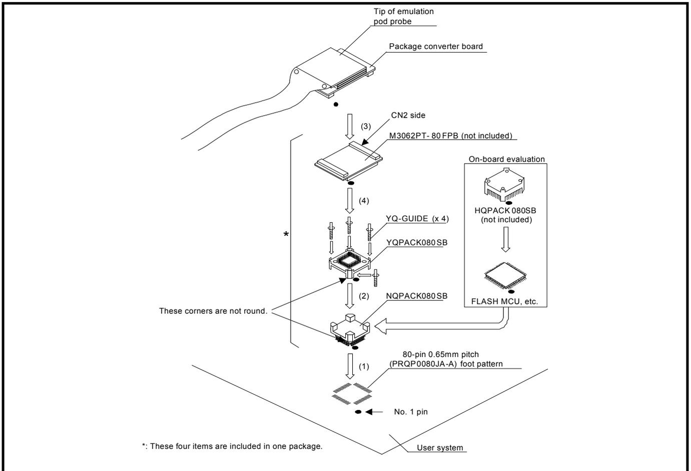
Figure 2.9 Connecting to a 80-pin 0.65mm pitch foot pattern
