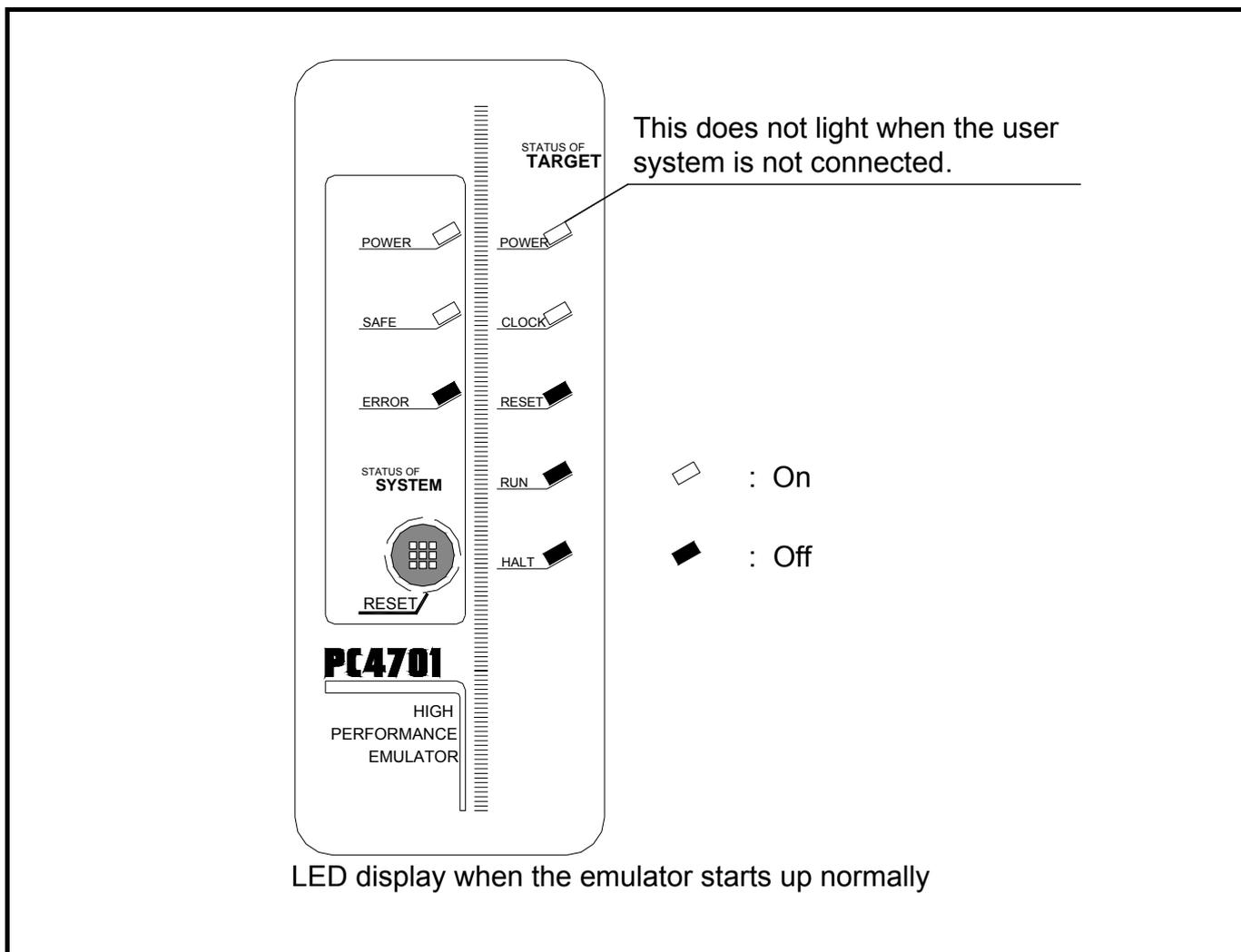
Figure 2.4 LED display when the power turned on
