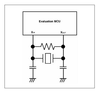
Figure 3.6 Circuit in which oscillation does not occur
