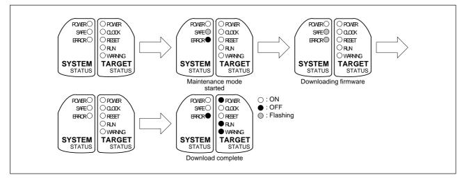
Figure 4.2 LEDs during firmware download
