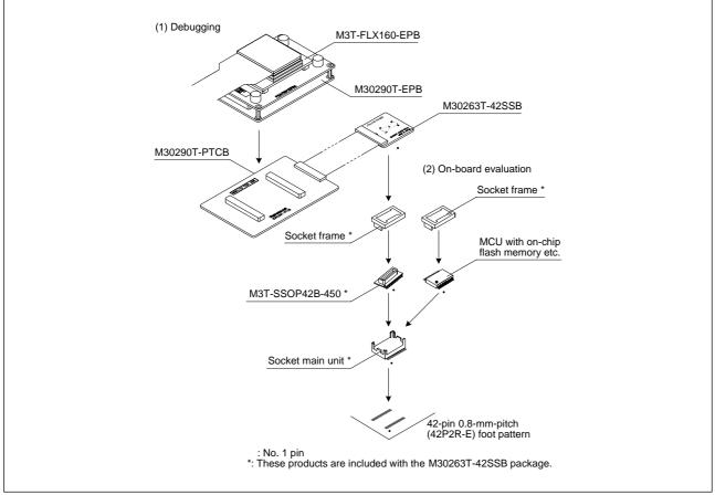
Figure 3.10 Connecting to a 42-pin 0.8-mm-pitch foot pattern
