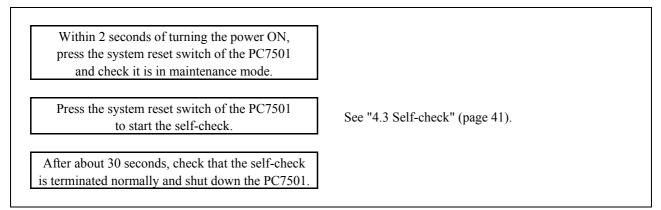
Figure 2.4 Self-check procedure
