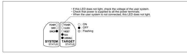
Figure 4.1 LED display of the PC7501 when the power turned on
