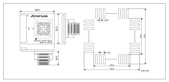
Figure 5.5 External dimensions and a sample foot pattern of the converter board M30291T-64FPD
