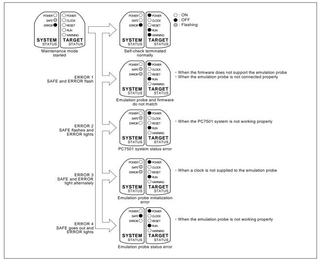
Figure 4.3 LED displays in the self-check
