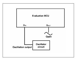
Figure 3.5 External oscillator circuit
