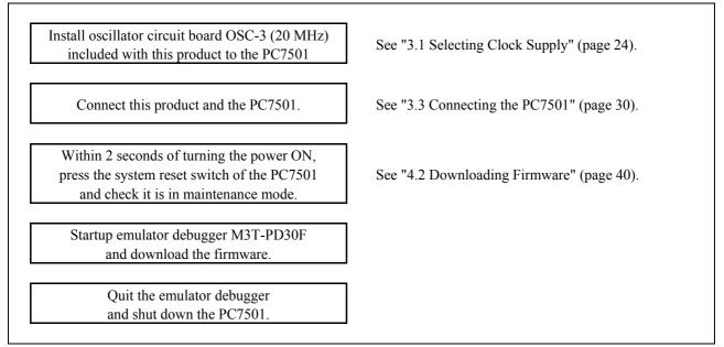
Figure 2.3 Firmware download procedure
