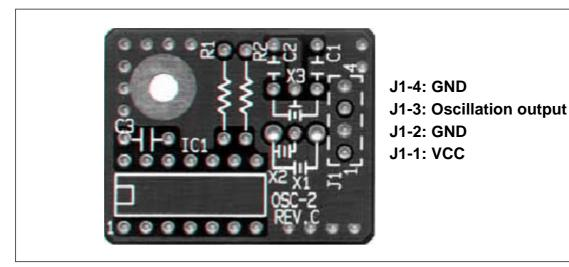
Figure 3.3 External view of the oscillator circuit board OSC-2 and its connector pin positions
