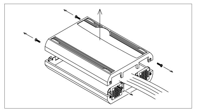
Figure 3.1 Removing the upper cover
