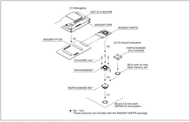
Figure 3.13 Connecting to an 80-pin 0.5-mm-pitch foot pattern
