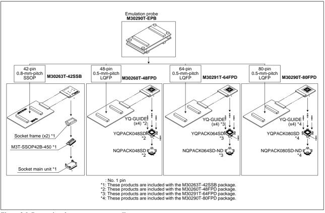
Figure 3.9 Connecting the user system according to user systems
