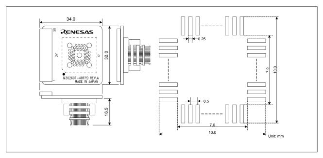
Figure 5.4 External dimensions and a sample foot pattern of the converter board M30260T-48FPD
