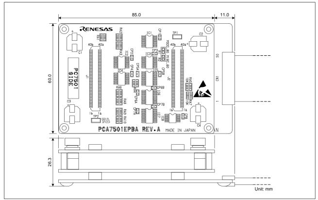
Figure 5.2 External dimensions of the emulation probe
