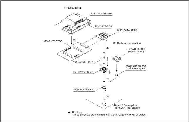
Figure 3.11 Connecting to a 48-pin 0.5-mm-pitch foot pattern
