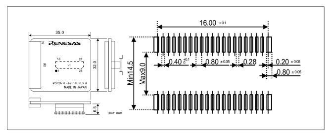
Figure 5.3 External dimensions and a sample foot pattern of the converter board M30263T-42SSB
