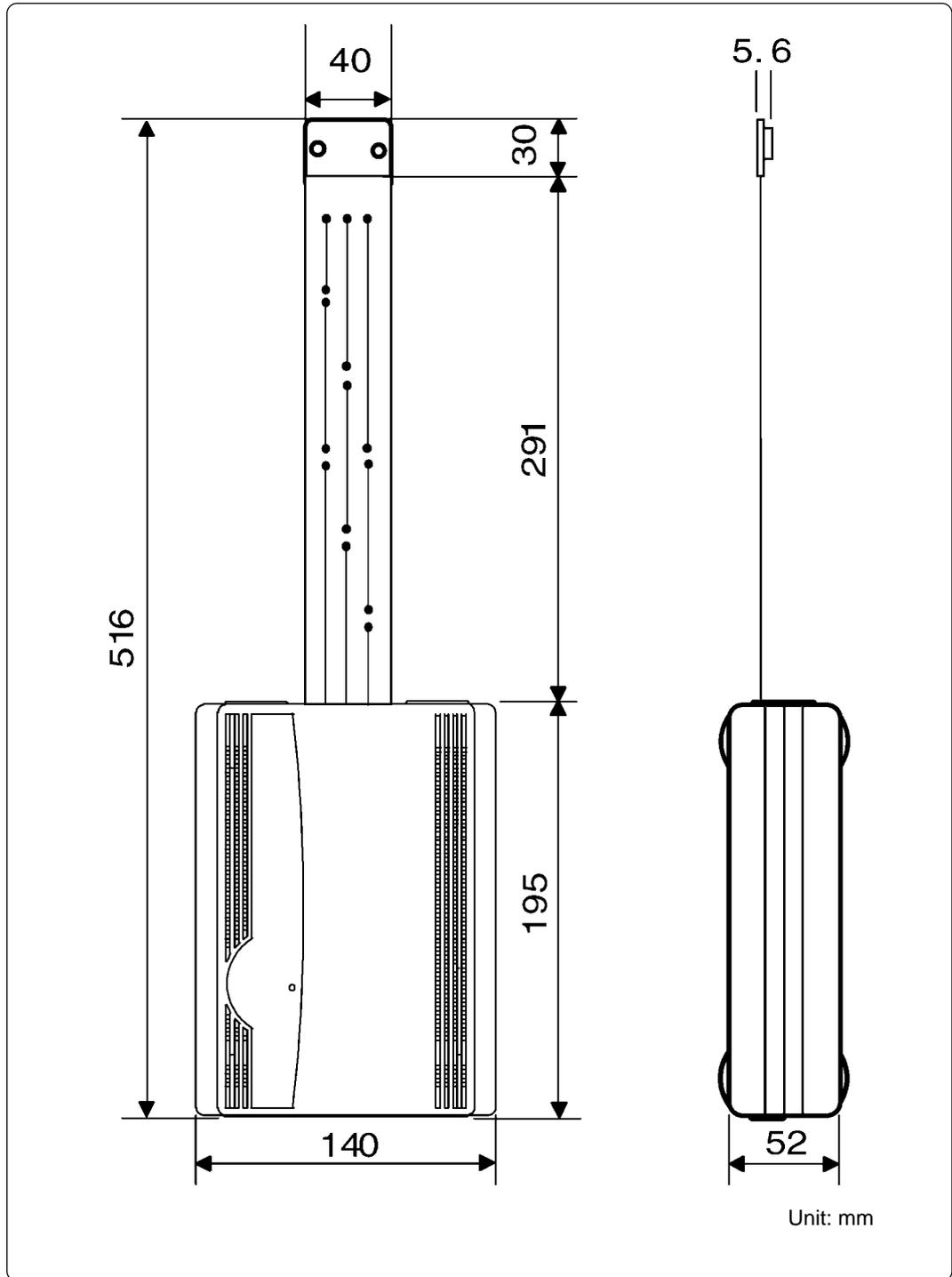
Figure 5.2 External dimensions of emulation pod
