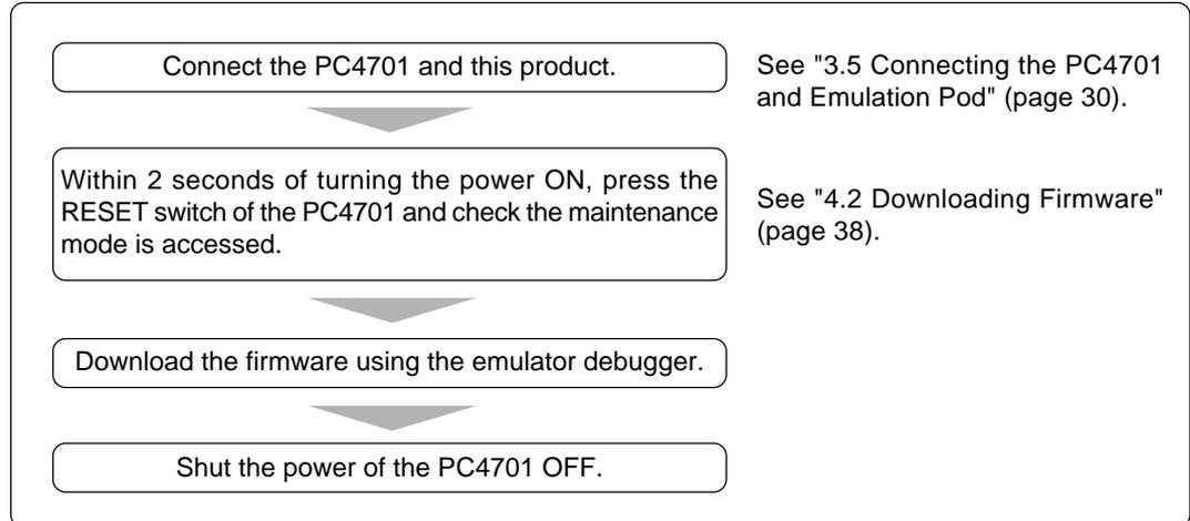
*Figure 2.3 Firmware download procedure when emulator is used for the first time*
