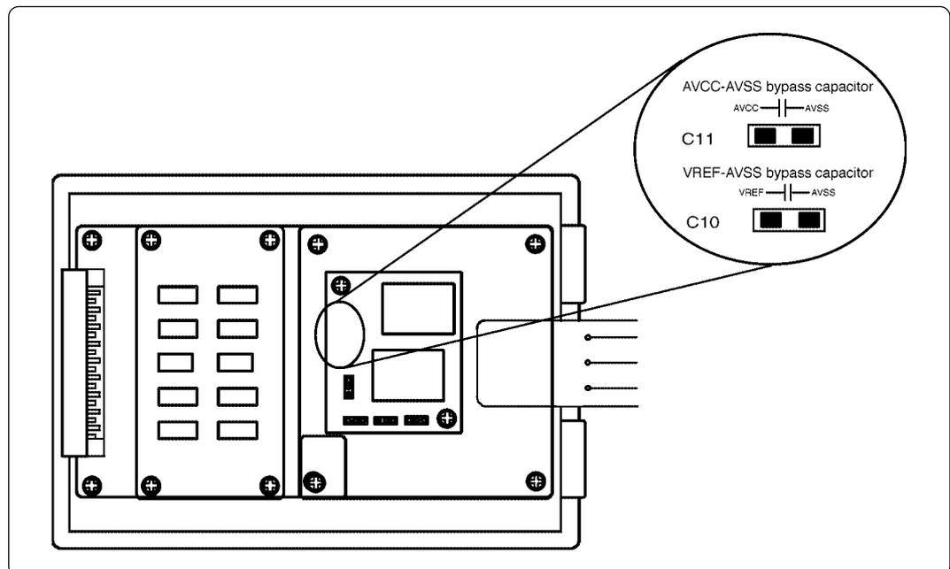
Figure 3.8 Foot patterns of A-D conversion bypass capacitor
