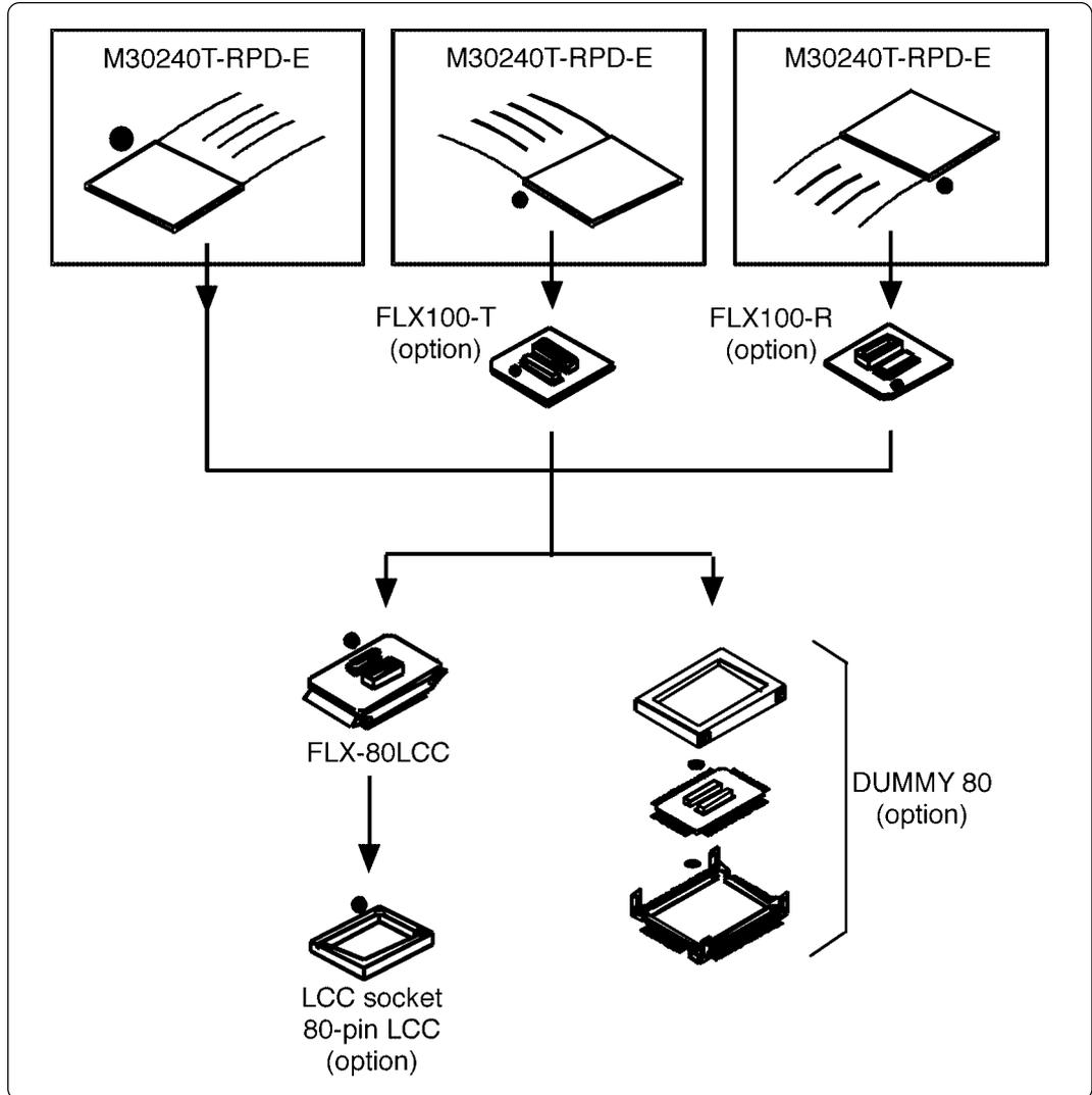
Figure 3.11 Connecting emulation pod and target systems
