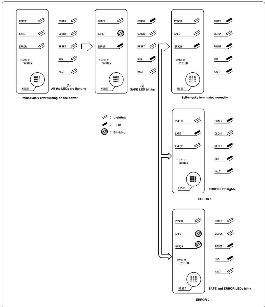
Figure 4.4 Self-check procedure
