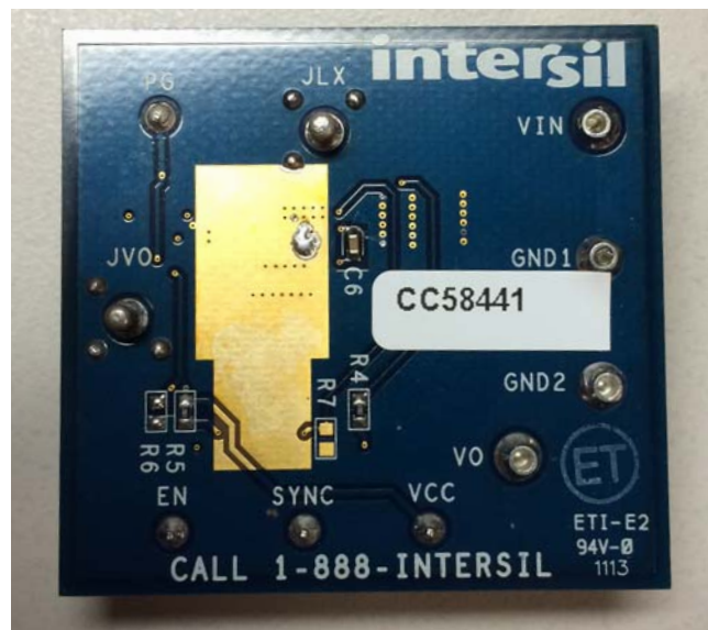
FIGURE 2. BACK OF EVALUATION BOARD ISL85413EVAL1Z
