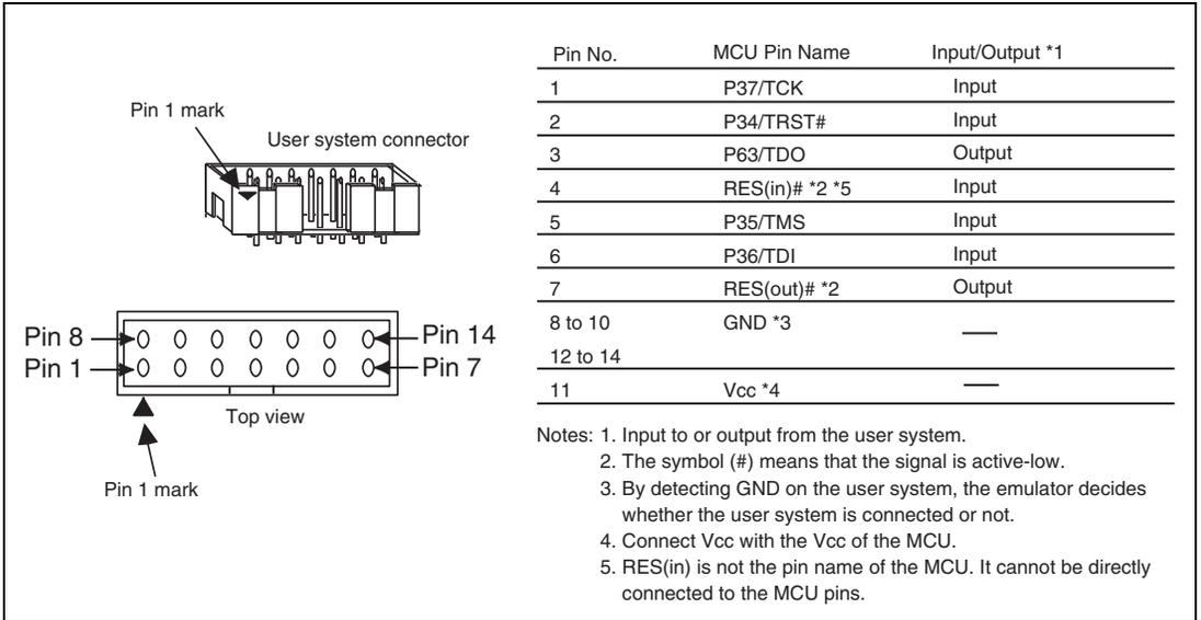
**Figure 1.2 Pin Assignments of the User System Connector**
