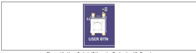
Figure 18. User Switch (S1) on the Evaluation Kit Board
