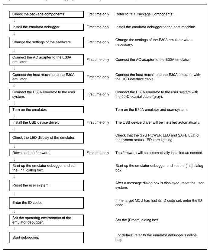
Figure 2.1 Flowchart of Starting the Debug
