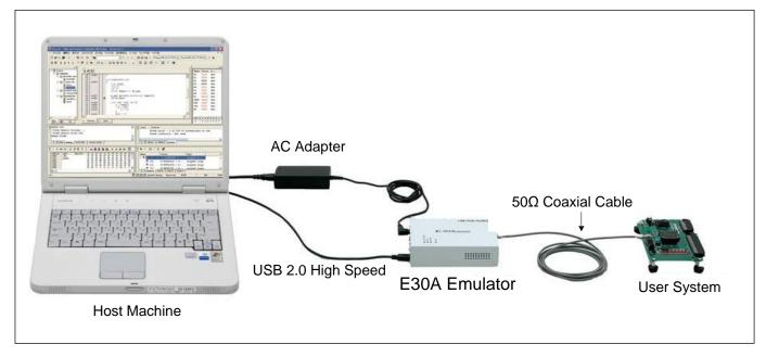
Figure 1.1 E30A Emulator System Configuration
