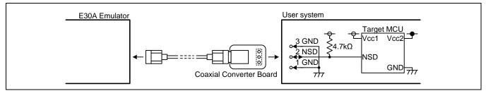
Figure 2.5 Connection Diagram when Using the Coaxial Converter Board
