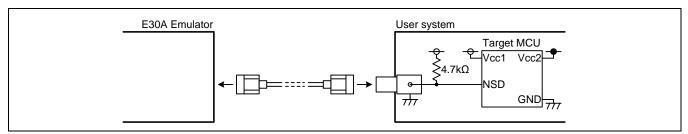
Figure 2.4 Connection Diagram when Using the Coaxial Connector
