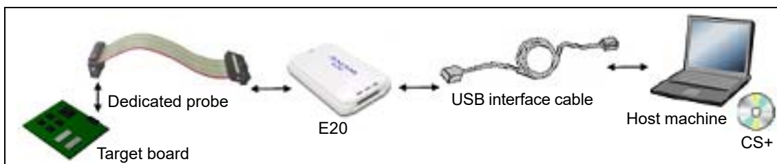
Figure 2.3 Connection Example [E20]
