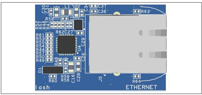
Figure 22. Ethernet Connector
