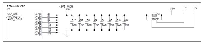
Figure 29. RA +3.3 V Current Measurement Circuit
