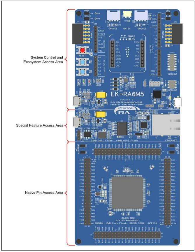
Figure 4. EK-RA6M5 Board Functional Area Definitions
