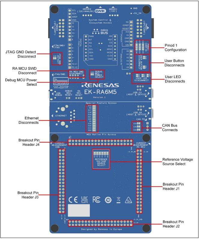
Figure 2. EK-RA6M5 Board Bottom Side
