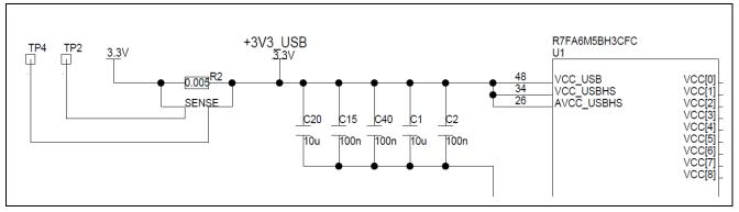
Figure 28. RA USB Current Measurement Circuit
