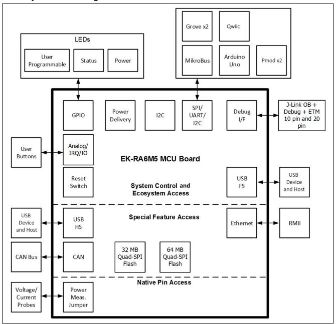
Figure 5. EK-RA6M5 Board Block Diagram
