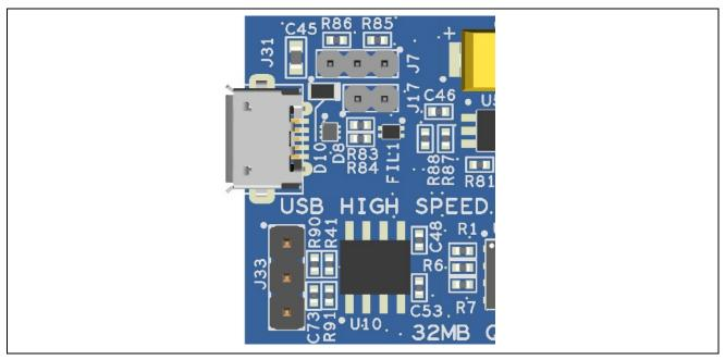
Figure 23. USB High Speed Connector
