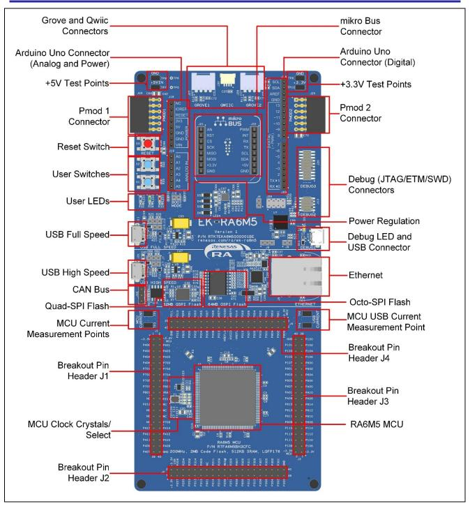
Figure 1. EK-RA6M5 Board Top Side
