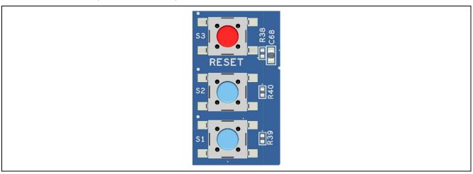
Figure 19. Reset and User Switches
