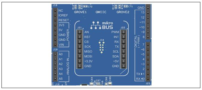
Figure 14. Arduino Uno Connectors
