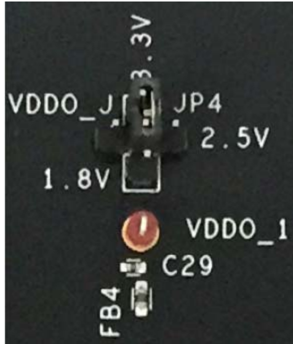
Figure 3. In the 4-way header, the central pin is the output and the other pins are 1.8V, 2.5V, 3.3V and VDDO_J (from J15) respectively. Jumper settings are selected according to the output voltage required for outputs 0, 1, 2 and 3.
