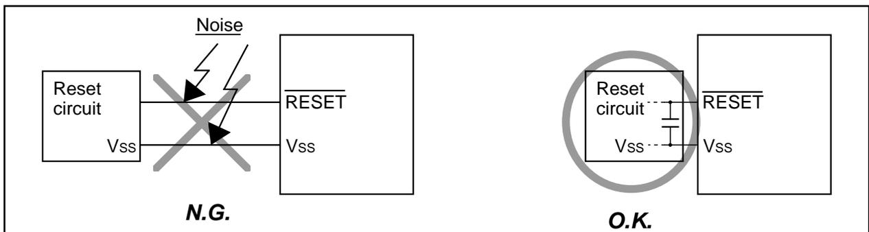
Figure 1.1.2. Wiring for  $\overline{\text{RESET}}$  pin
