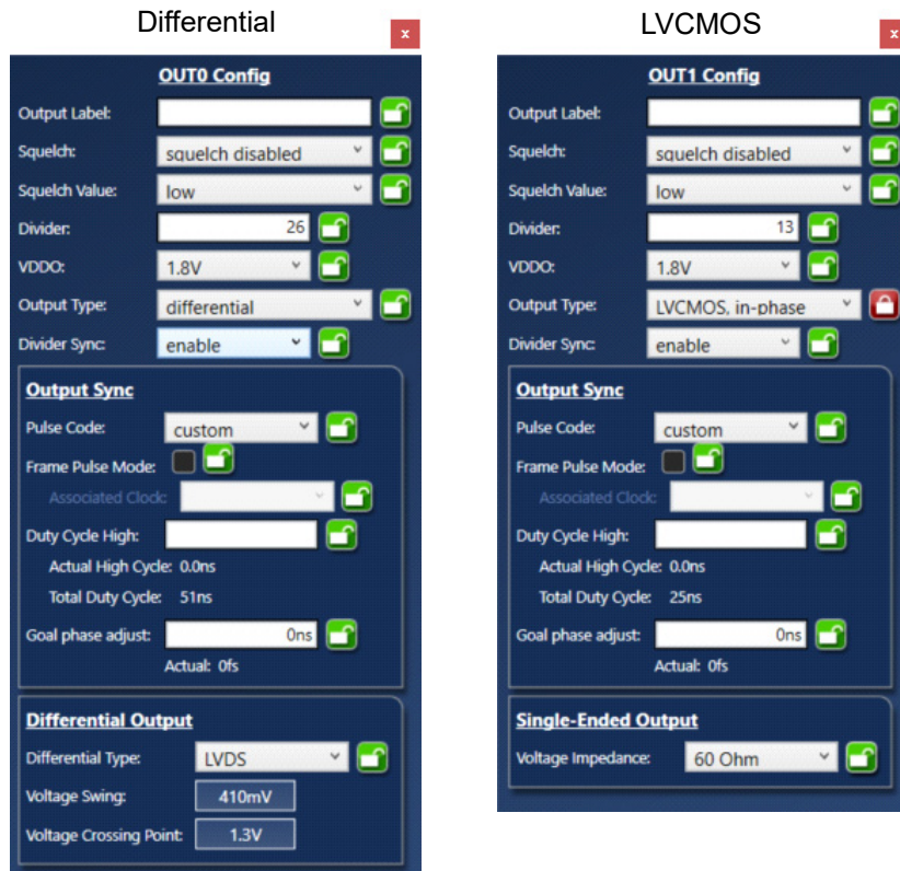
Figure 15. Output Stages – Differential and LVCMOS Signals Windows
