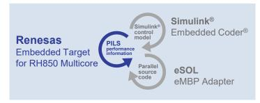
Embedded Target for RH850 Multicore is a MATLAB® collaborative environment that automatically generates parallel codes and a Processor In the Loop Simulation (PILS) environment from a Simulink® model. This development environment also supports automatic multicore allocation in corporation with the model based parallelizer of eSOL Co., Ltd.
