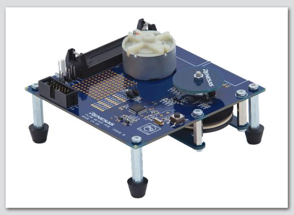
The sensor disk's RPM may be controlled by tuning the motor's DC voltage. An optical sensor is included to determine the exact RPM of the disk.
