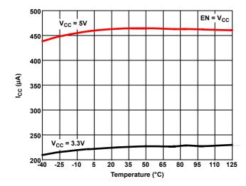
Figure 12. Supply Current vs Temperature
