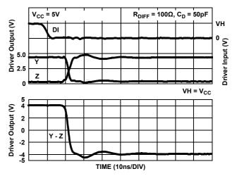
Figure 19. Driver Waveforms, High to Low
