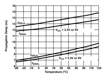
Figure 14. Driver Differential Propagation Delay vs
