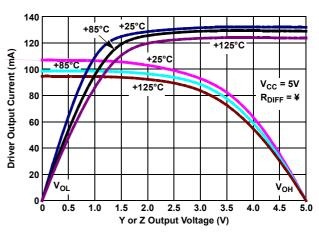
Figure 11. Driver Single-Ended (Y or Z) Output Current vs Output Voltage
