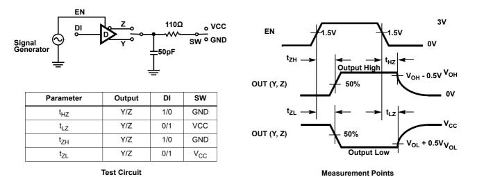
Figure 6. Driver Enable and Disable Times
