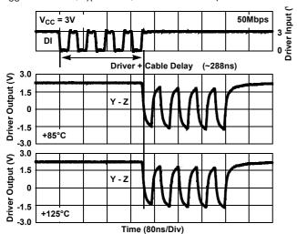
Figure 20. Worst Case (Negative) Five Pulse Driver Waveforms Driving 200 Feet (62m) of Cat5 Cable (Single Terminated with  $121\Omega$ )
