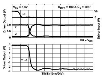
Figure 17. Driver Waveforms, High to Low
