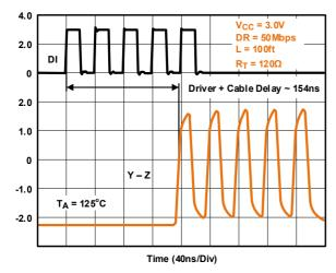
Figure 1. Data Rate Performance at 3.0V
