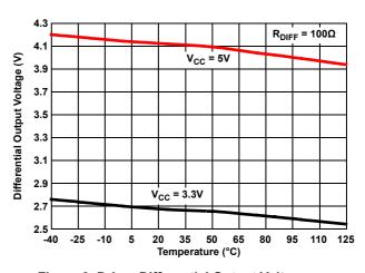
Figure 9. Driver Differential Output Voltage vs
