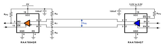
Figure 3. Network Using Group Enables
