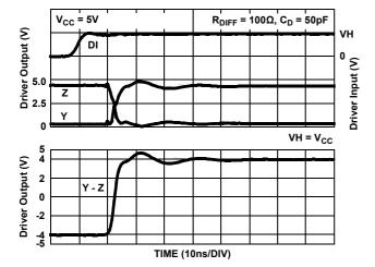
Figure 18. Driver Waveforms, Low to High
