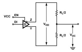
**Figure 4. DC Driver Test Circuits**
