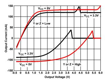
Figure 13. Driver Output Current vs Short-Circuit Voltage
