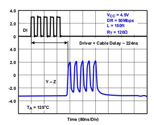
Figure 2. Data Rate Performance at 4.5V
