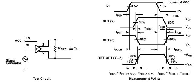
Figure 5. Driver Propagation Delay and Differential Transition Times
