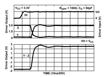
Figure 16. Driver Waveforms, Low to High
