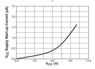
Figure 8.5 :  $V_{\text{CC}}$  vs.  $V_{\text{CC}}$  Supply Start-up Current
