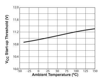
Figure 8.2 : Start-Up Threshold vs. Temperature
