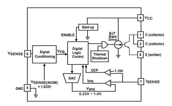
Figure 9.1: iW1816 Functional Block Diagram
