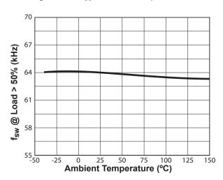
Figure 8.3 : Switching Frequency vs. Temperature
