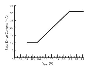
Figure 10.5 : Base Drive Current vs. VIPK
