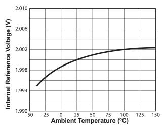
Figure 8.4 : Internal Reference vs. Temperature
