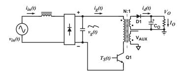
Figure 10.2 : Simplified Flyback Converter
