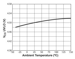
Figure 8.1 : V<sub>CC</sub> UVLO vs. Temperature
