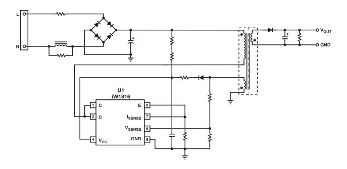
Figure 3.1: iW1816 Typical Application Circuit
