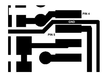
FIGURE 14. LAYOUT DETAIL OF GND BETWEEN PINS 4 AND 5
