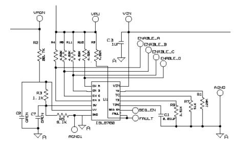
FIGURE 15. ISL870xEVAL1 PHOTOGRAPH AND SCHEMATIC OF LEFT CHANNEL
