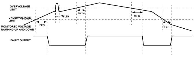
FIGURE 3. ISL8702 FAULT OPERATIONAL DIAGRAM
