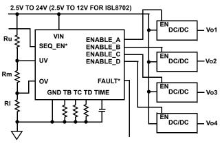
\* SEQ\_EN and FAULT are not available on ISL8700 and ISL8701 FIGURE 1. ISL870x IMPLEMENTATION
