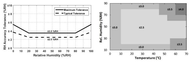
Figure 4. HS41x3 RH Accuracy Tolerance at 25°C
