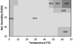
Figure 3. HS41x1 RH Accuracy over Temperature
