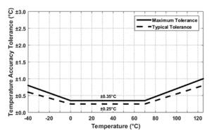
Figure 7. HS41x3 Temperature Sensor Accuracy Tolerance
