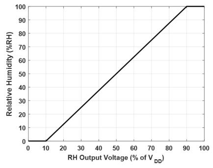
Figure 9. Relative Humidity vs. VRH Output Analog Voltage
