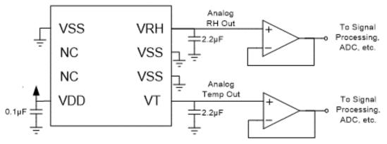
Figure 8. HS41xx Application Circuit
