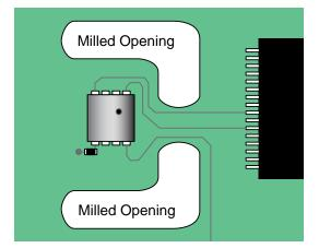
Figure 12. Milled PCB Openings for Thermal Isolation
