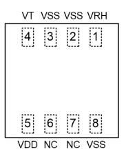
Figure 1. Pin Assignments – Top View
