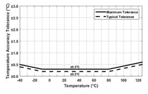
Figure 6. HS41x1 Temperature Sensor Accuracy Tolerance
