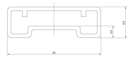
MM525-02A, LB-066 Length: 500±2.0 Thickness: 0.8<sup>+0.3</sup><sub>-0.2</sub> Tolerance: ±0.4
