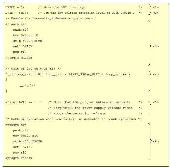
**[Example 2]** Using the low-voltage detection function as an interrupt by setting the low-voltage detection level  $(V_{LVI})$  to 2.95 V (TYP.)  $\pm$  0.10 V.
