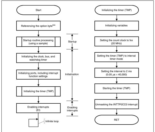
**Note** The option byte is automatically referenced by the microcontroller after a reset is released. In this sample program, the oscillation stabilization time after releasing reset is set to 6.554 ms with the option byte.
