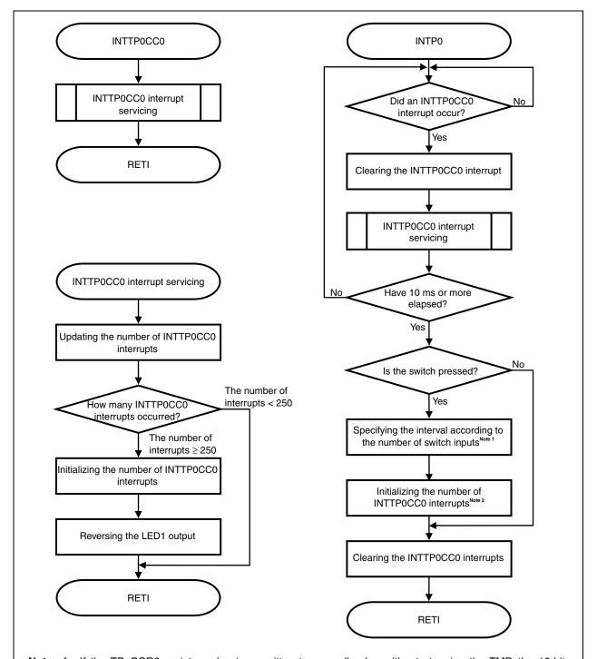
Notes 1. If the TPnCCR0 register value is re-written to a small value without stopping the TMP, the 16-bit counter might overflow. For details, see the user's manual.
