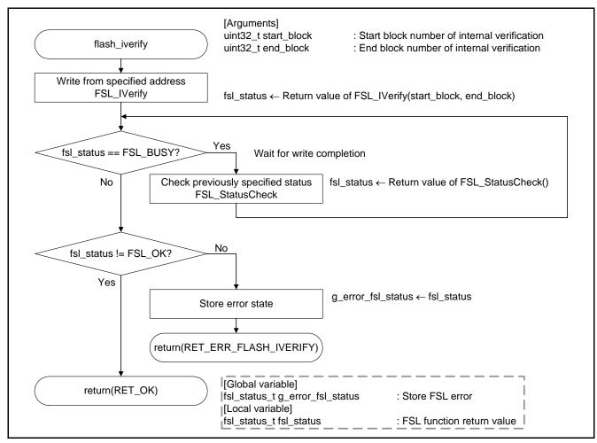
Figure 6.17 Internal Verification of Specified Block
