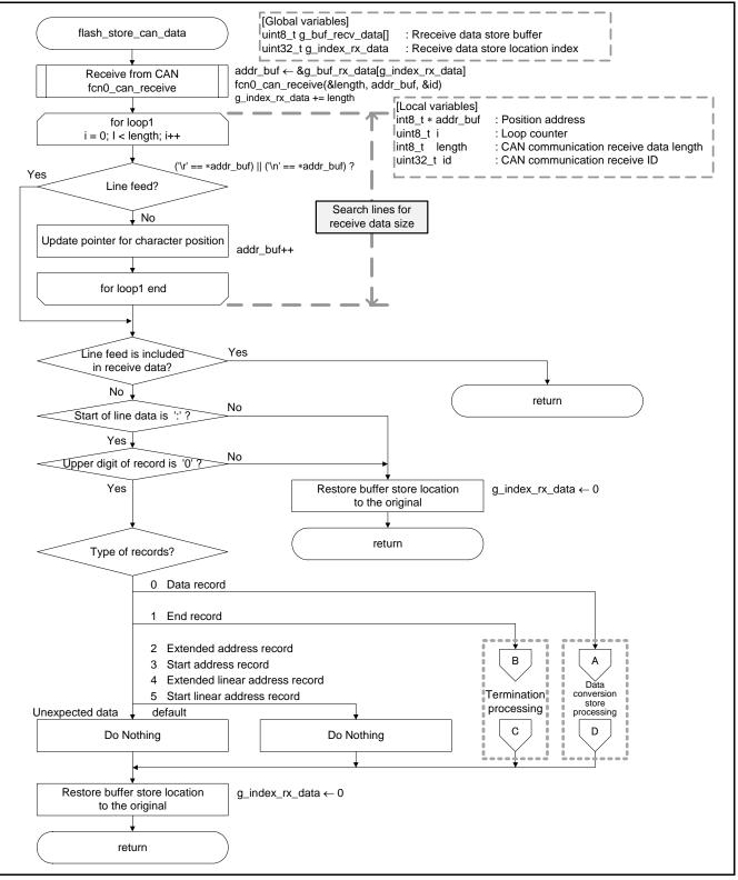
Figure 6.20 Store Processing for Receive Data (1/2)
