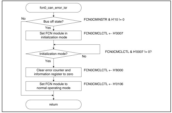
Figure 6.33 FCN0 Error Interrupt Processing
