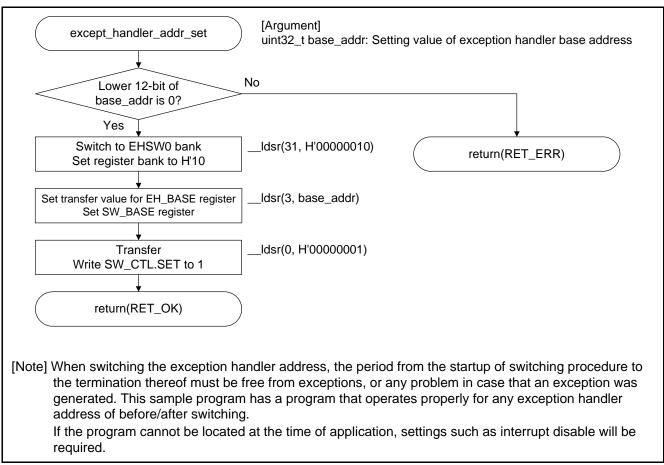
Figure 6.6 Switching Processing for Exception Handler Address
