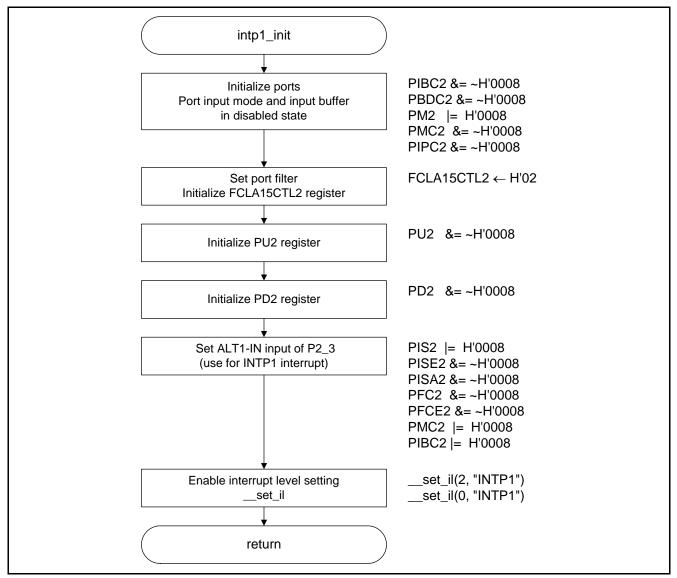
Figure 6.8 Initialization of INTP1 Interrupt
