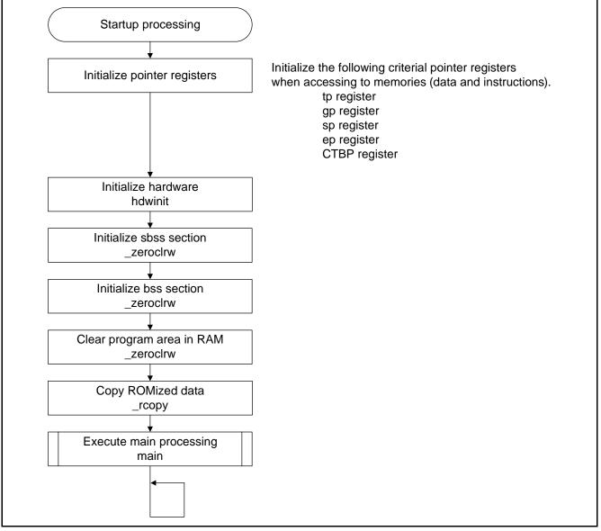
Figure 6.4 Startup Routine Processing
