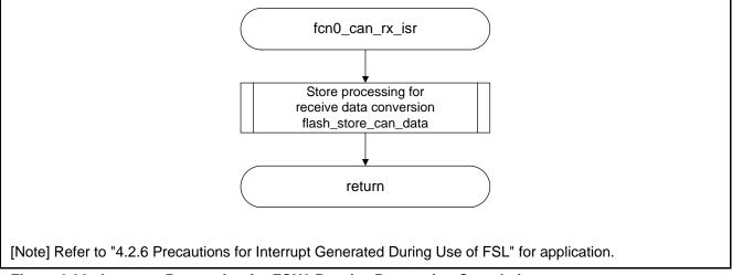
Figure 6.32 Interrupt Processing for FCN0 Receive Processing Completion
