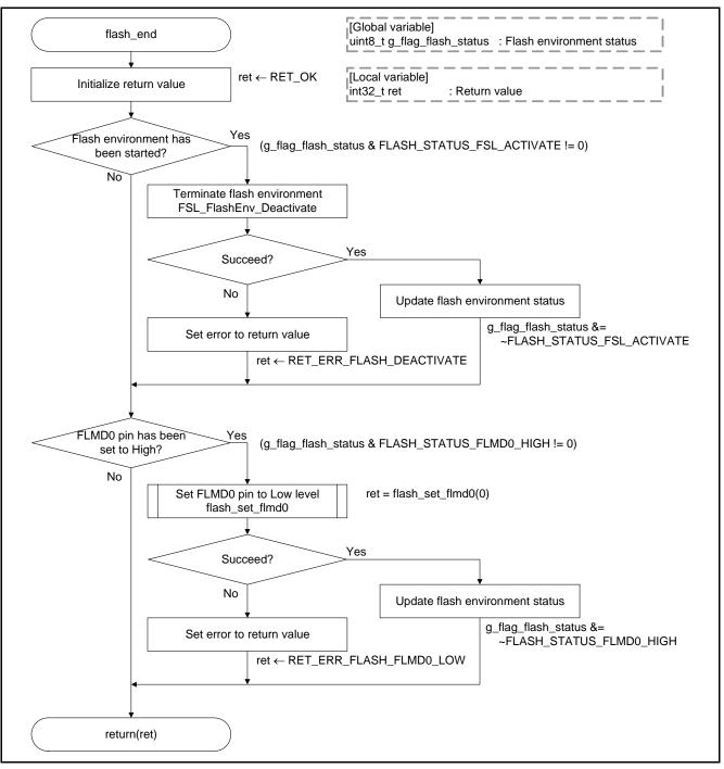
Figure 6.18 Termination Processing for Flash Environment
