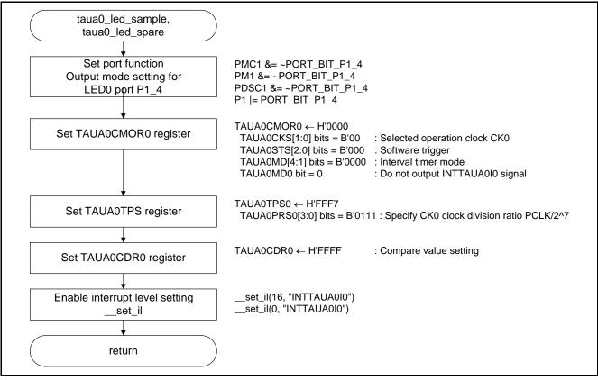
Figure 6.23 TAUA0 Initialization for LED Flash with Fixed-Cycle
