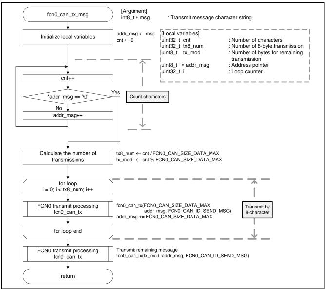
Figure 6.29 FCN0 Message Transmit Processing
