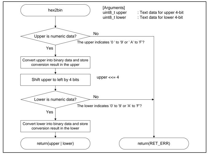
Figure 6.22 Text Binary Conversion Processing
