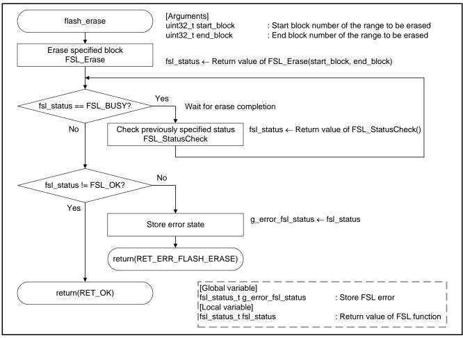
Figure 6.15 Erase Processing for Specified Block
