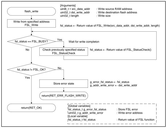
Figure 6.16 Write Processing from Specified Address
