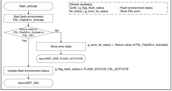
Figure 6.13 Start Processing for Flash Environment
