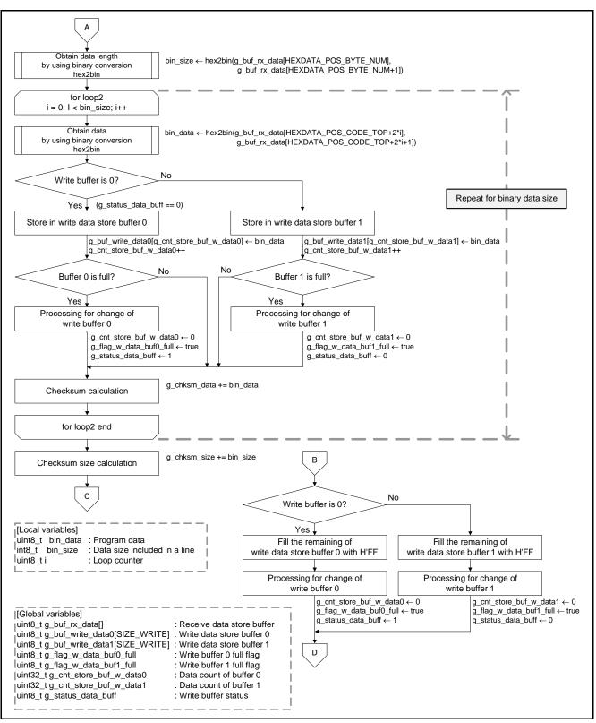
Figure 6.21 Store Processing for Receive Data (2/2)
