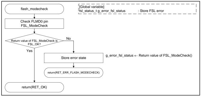
Figure 6.14 Checking Processing for FLMD0 Pin using FSL
