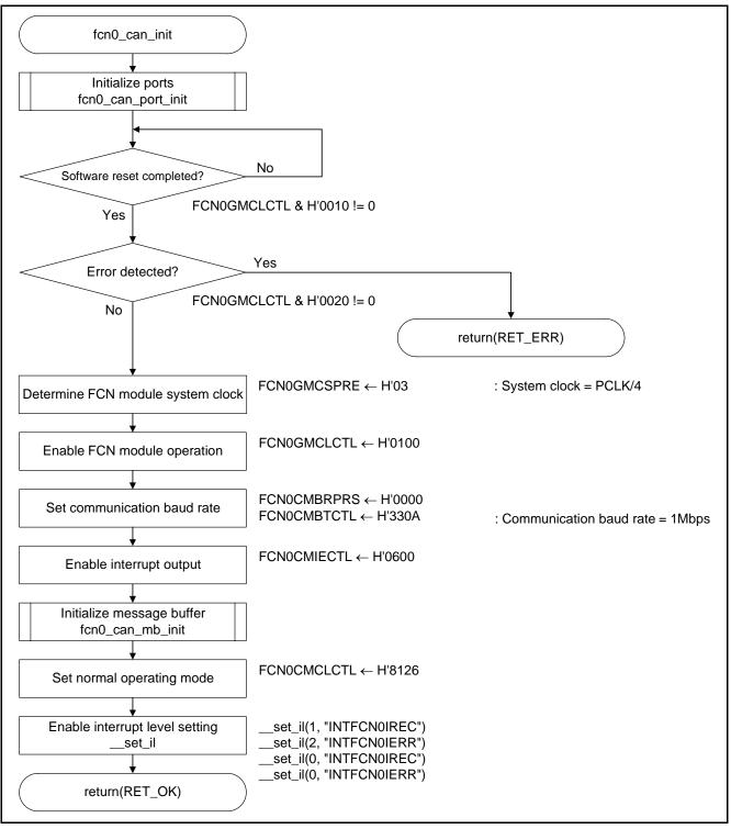
Figure 6.25 Initialization of CAN Controller Channel 0 (FCN0)
