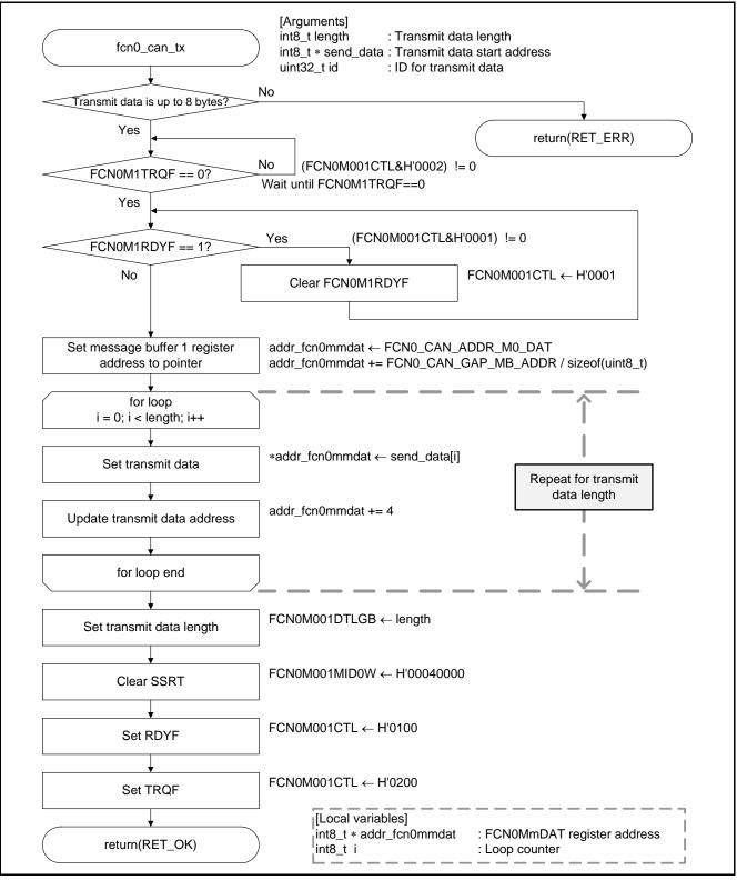
Figure 6.30 FCN0 Transmit Processing
