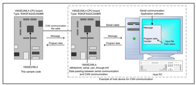
Figure 7.1 Hardware Configuration Example for Sample Code
