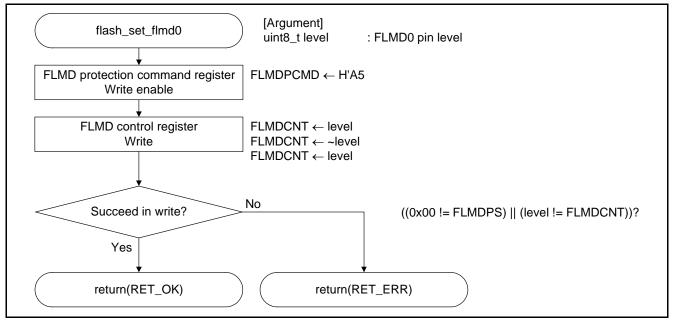
Figure 6.19 Setting for FLMD0 Pin Level
