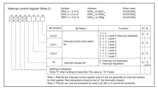
**Figure 7 Timer Interrupt Control Register**
