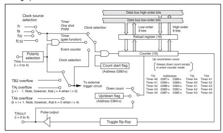
Figure 1 Bock Diagram of Timer A
