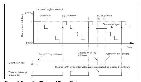
**Figure 3 Operation Timing of Timer Mode**
