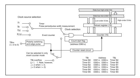
Figure 2 Block Diagram of Timer B
