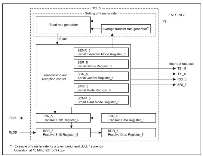
Figure 3 SCI\_5 Block Diagram
