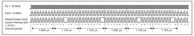
Figure 8 Example of Internal-Base-Clock Generation When Pf = 16 MHz and ACS3 to 0 = B'0011
