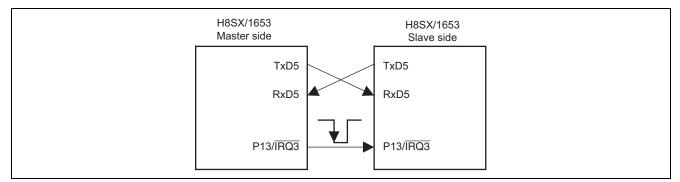
Figure 1 Setup for Asynchronous Communications with Timing from the Average Transfer Rate Generator
