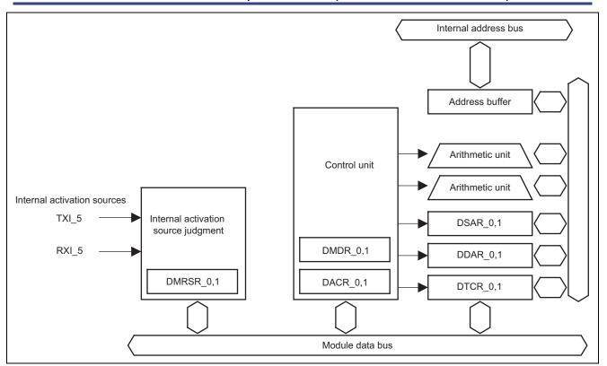
Figure 4 DMAC Block Diagram
