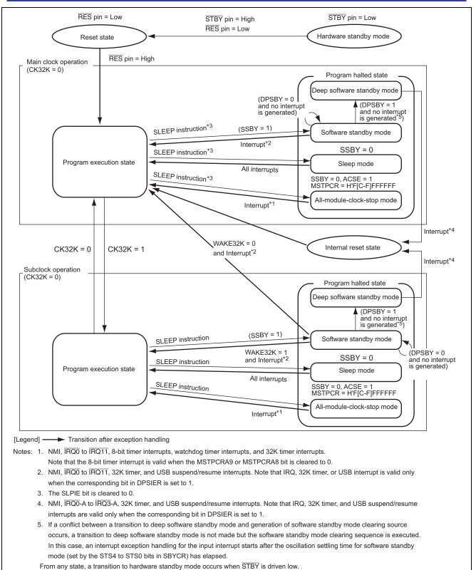
From any state except hardware standby mode, a transition to the reset state oc curs when RES is driven low.
