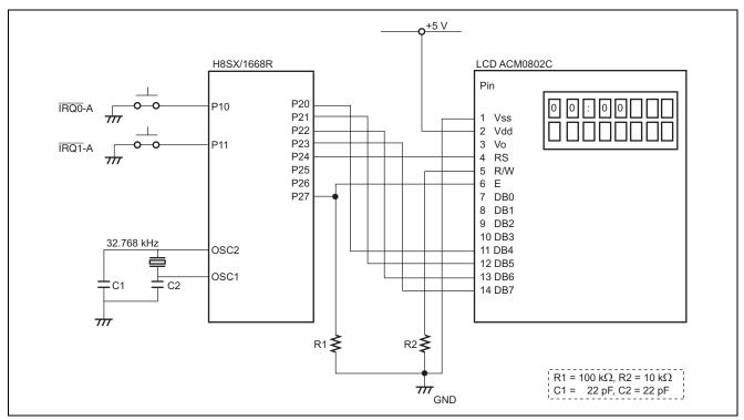
Figure 1 Configuration of the 24-Hour Clock
