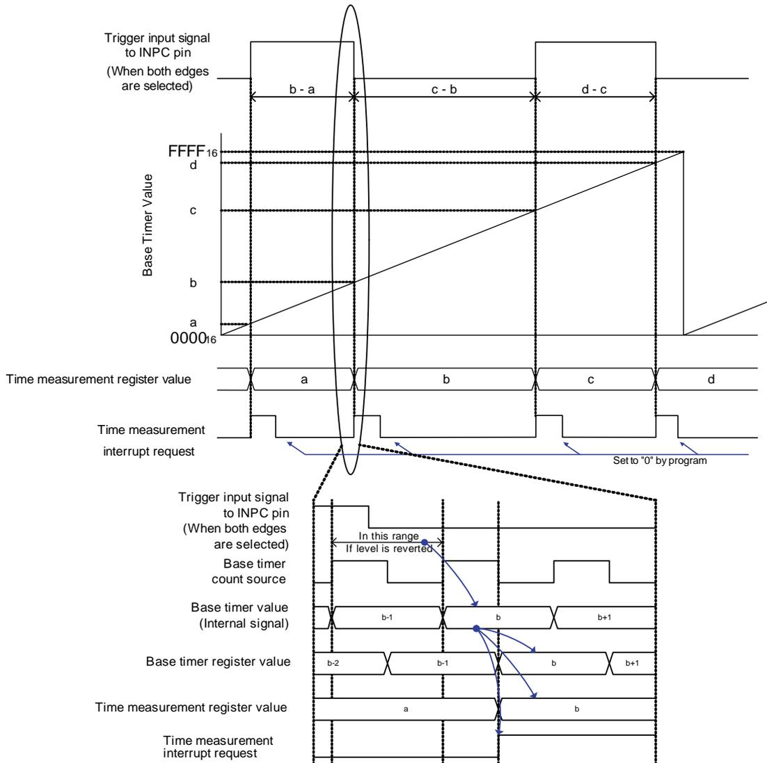
**Figure 2 Operation Timing of Time Measurement Function**
