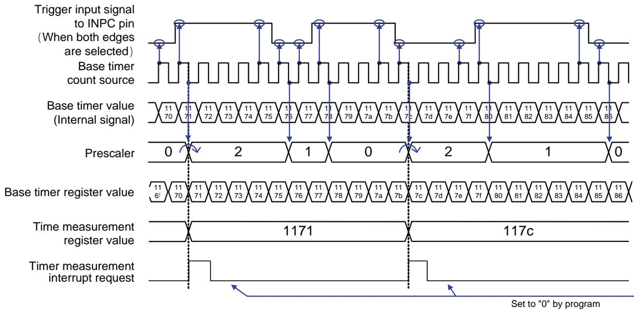
**Figure 6 Prescaler Operation Timing Diagram**
