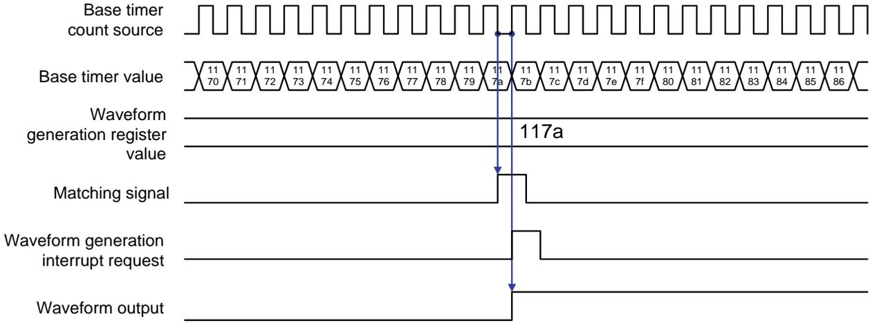
Figure 7 Waveform Generation Output Function (Output Compare) Operation Timing
