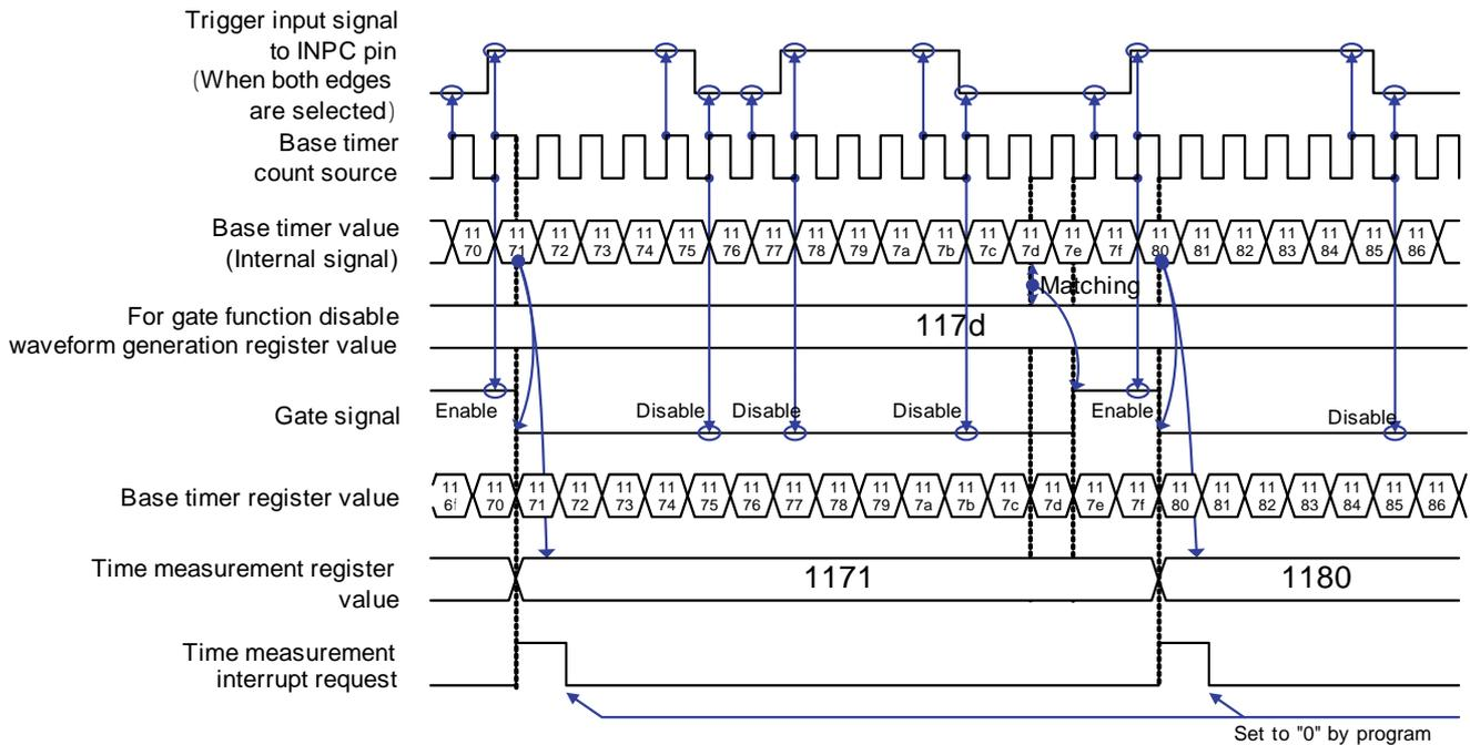
Figure 5 Gate Function Operation Timing Diagram
