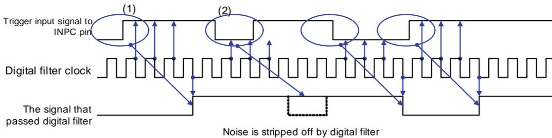
Figure 4 Digital Filter Operation Timing
