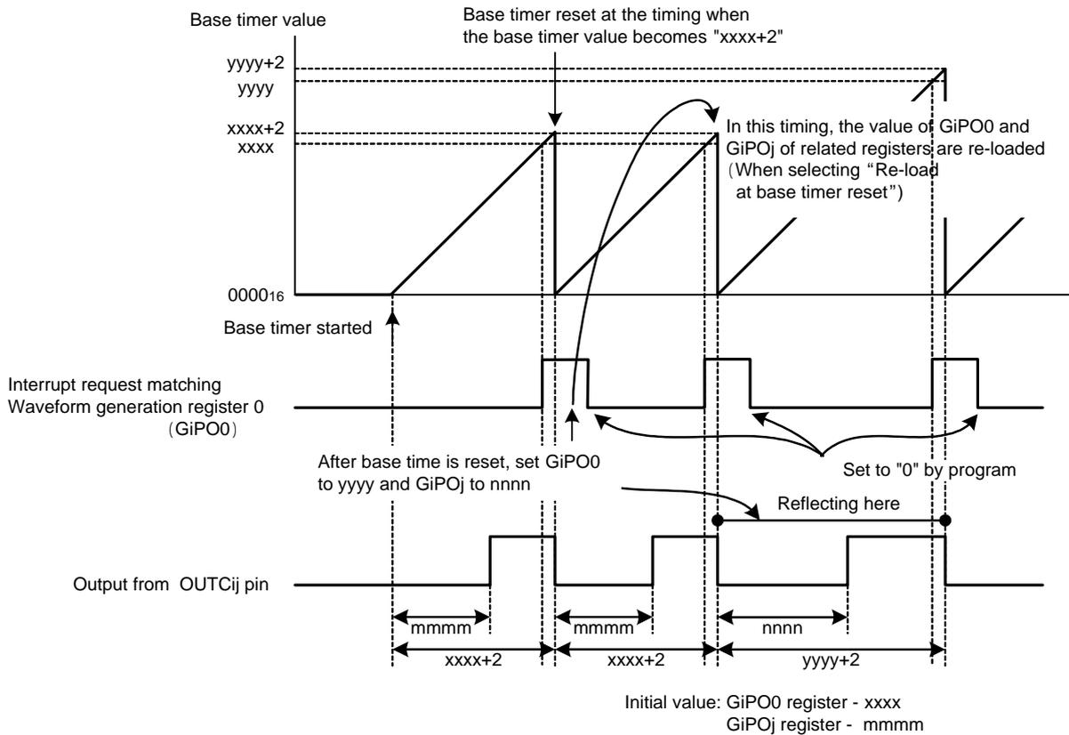
Figure 10 16-bit PWM Output Diagram
