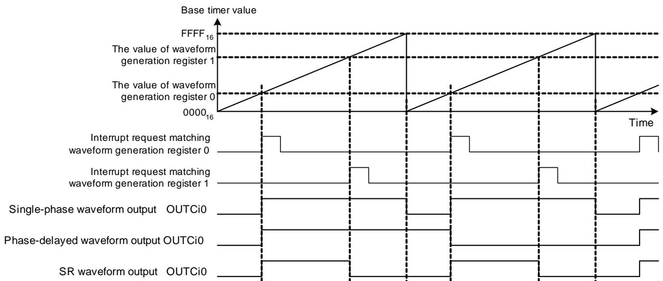
Figure 8 Waveform Generation Output Operation Timing
