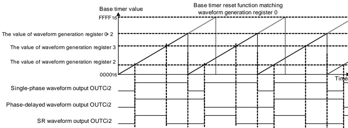
**Figure 9 Base Timer Reset Operation Diagram**
