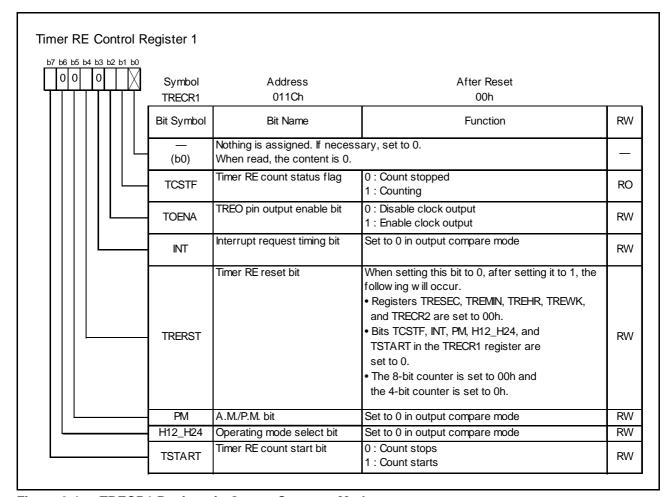
Figure 3.4 TRECR1 Register in Output Compare Mode
