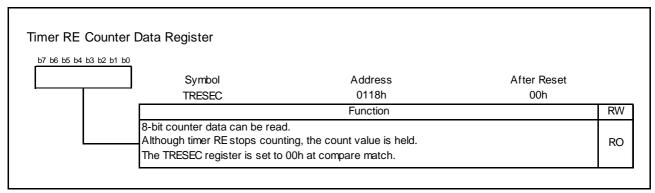
Figure 3.2 TRESEC Register in Output Compare Mode
