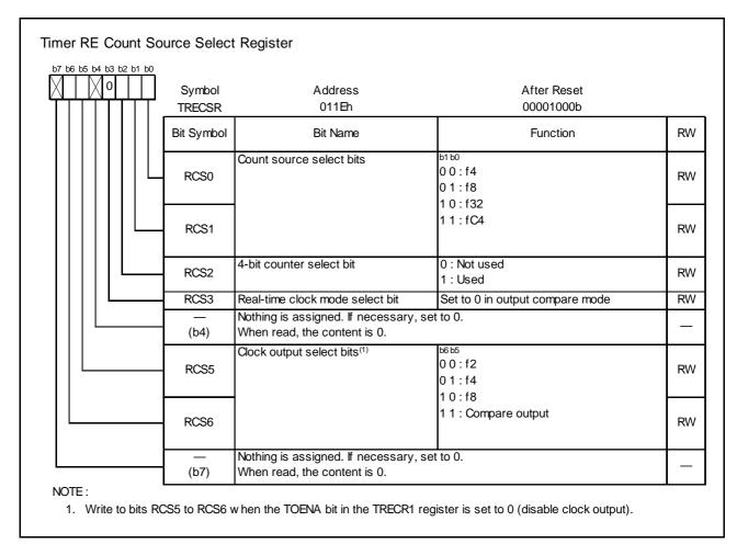
Figure 3.6 TRECSR Register in Output Compare Mode
