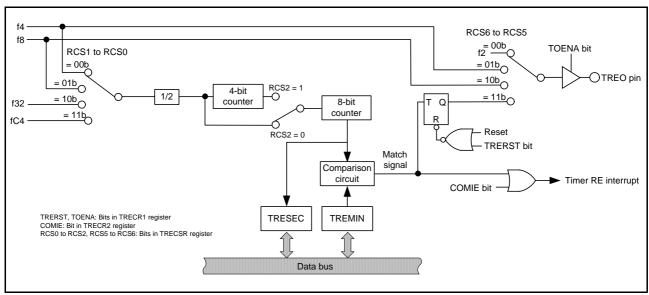
Figure 3.1 Block Diagram of Output Compare Mode
