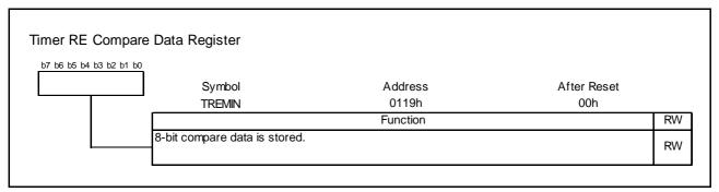
Figure 3.3 TREMIN Register in Output Compare Mode
