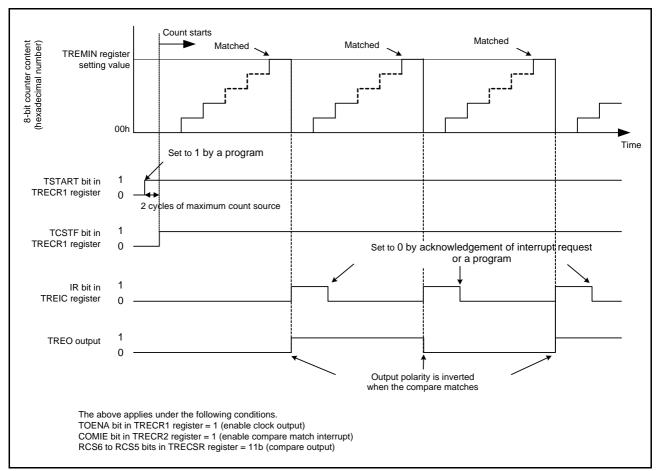
Figure 3.7 Operation in Output Compare Mode
