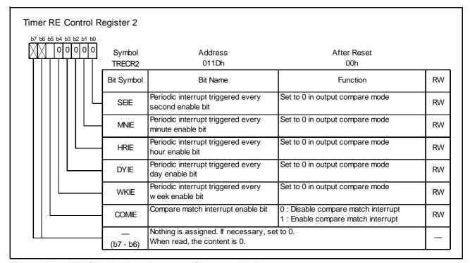
Figure 3.5 TRECR2 Register in Output Compare Mode
