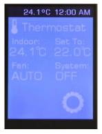
3. Tap the settings icon (looks like a gear) on the bottom right to make adjustments to the system including Units, Time and Date.
