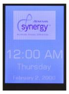
2. Tap the splash screen to enter the Thermostat demo. In this demonstration, the SSP uses the A/D converter to read the internal temperature sensor of the S7G2 and display this information on the LCD Display.
