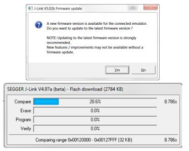
Jlink is programing the SK-S7G2 with the Out-Of-Box Demo
