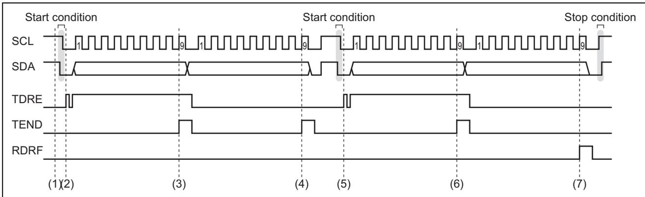
Figure 5 Timing of Operations in Master Transmit Mode
