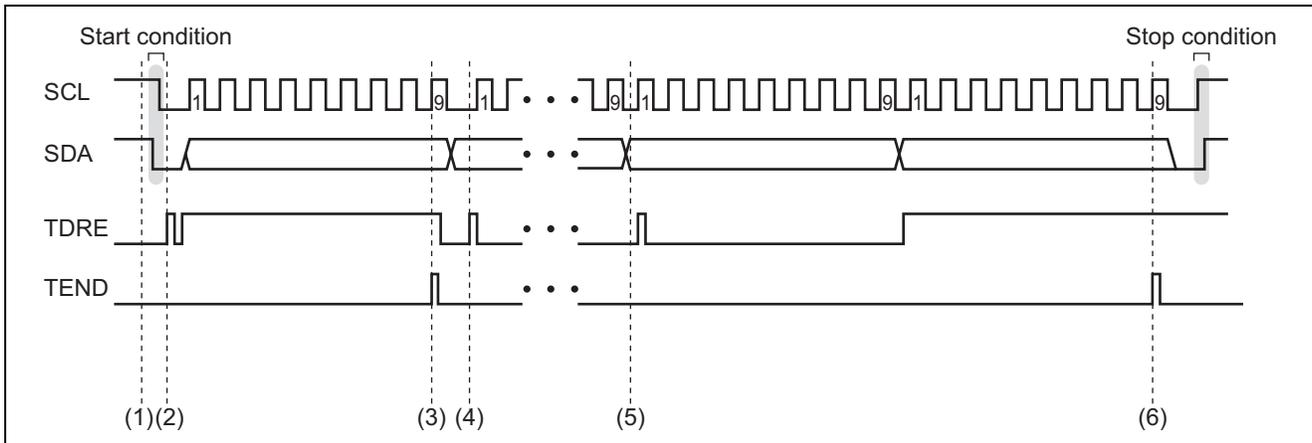
**Figure 2 Timing of Operations in Master Transmit Mode**
