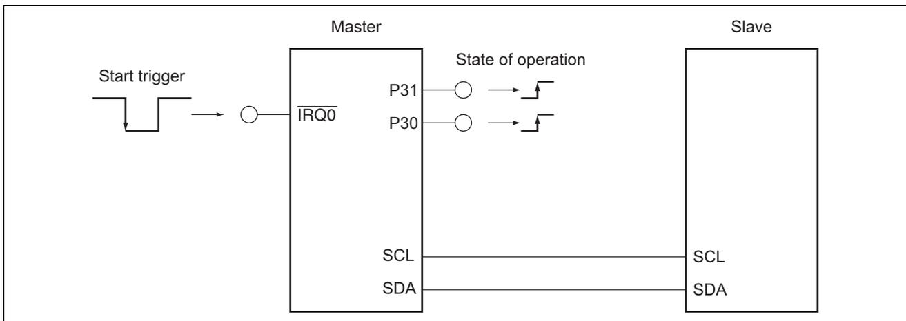
**Figure 1 Connections for I<sup>2</sup>C Bus Interface 2 Single-Master Mode Communication**
