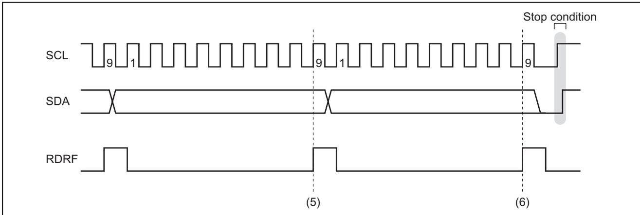
**Figure 4 Timing of Operations in Master Receive Mode 2**
