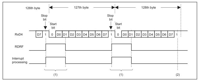
Figure 5 Receive Operation Timing
