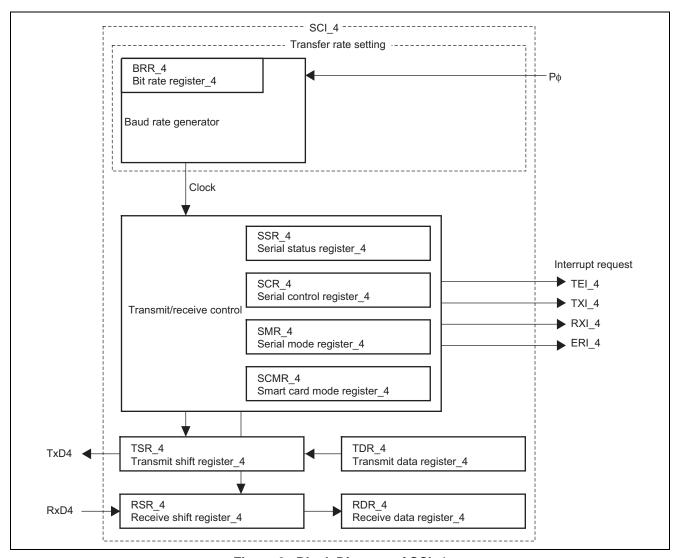
Figure 2 Block Diagram of SCI\_4
