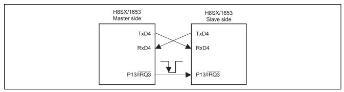
Figure 1 Connection for Simultaneous Transmission and Reception by SCI in Asynchronous Mode
