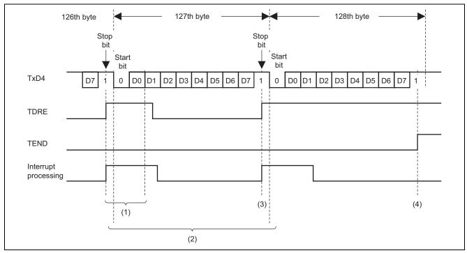
Figure 4 Transmit Operation Timing
