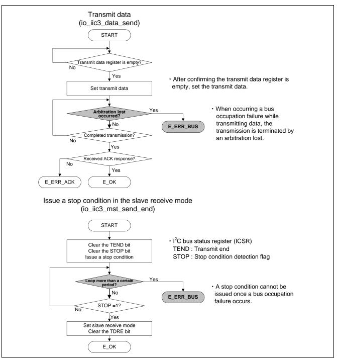
Figure 6.8 Functions for Data Transmission
