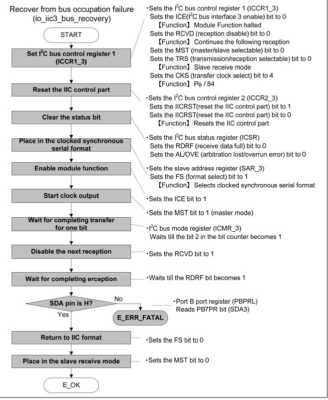
Figure 6.9 Function for Recovery from Bus Occupation State
