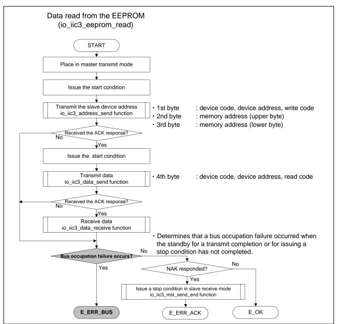
Figure 6.4 Function for Data Read from EEPROM
