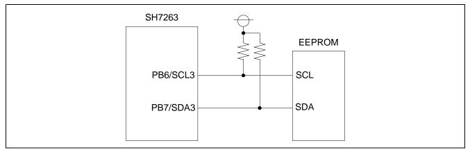
Figure 5.1 Configuration Diagram
