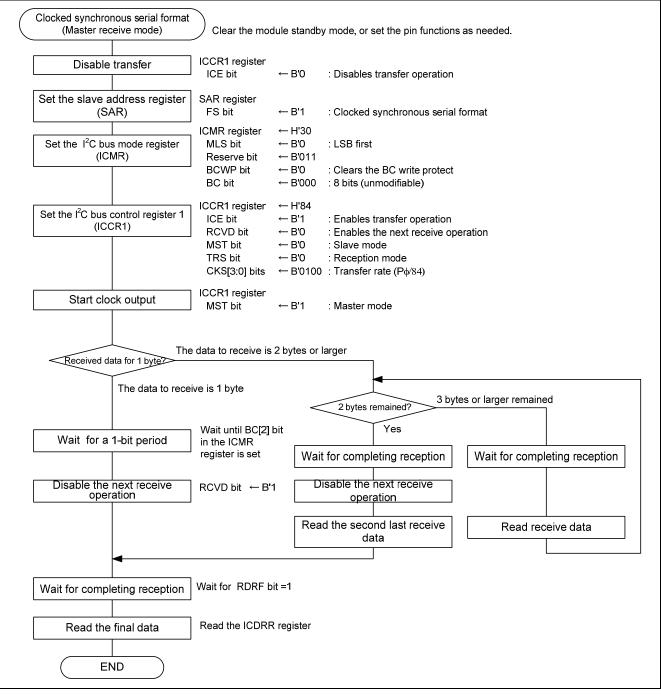
Figure 4.1 Setting Master Receive Mode in Clocked Synchronous Serial Format (Example)
