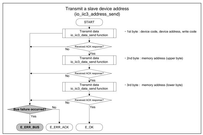
Figure 6.7 Function for Slave Device Address Transmission
