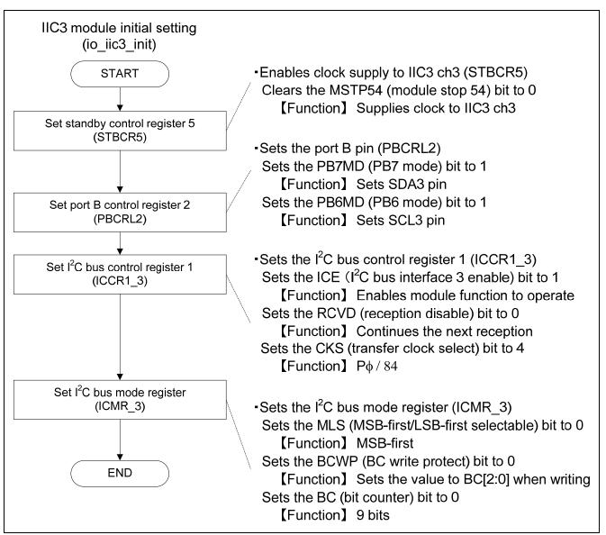
Figure 6.3 IIC3 Module Initialization
