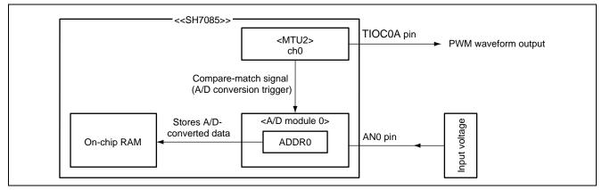
Figure 1 Block Diagram of A/D Conversion Controlled by MTU2
