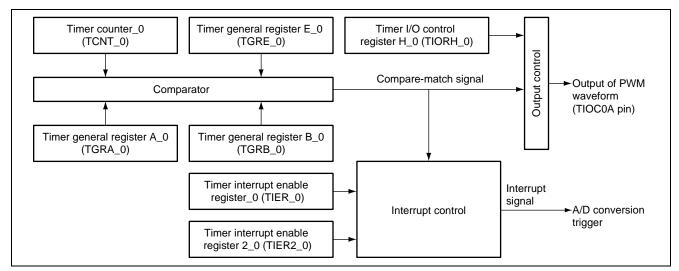
Figure 3 Block Diagram of MTU2 ch0
