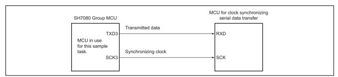
Figure 1 SCIF Serial Data Transmission in the Clock Synchronous Mode
