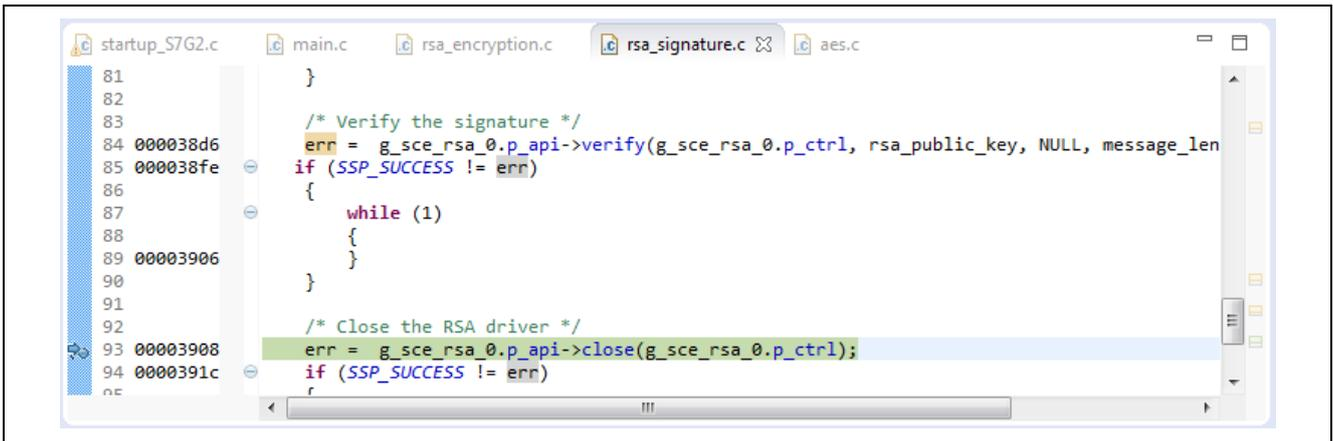
Figure 11 Breakpoint placed after signature verification in “rsa\_signature.c” file
