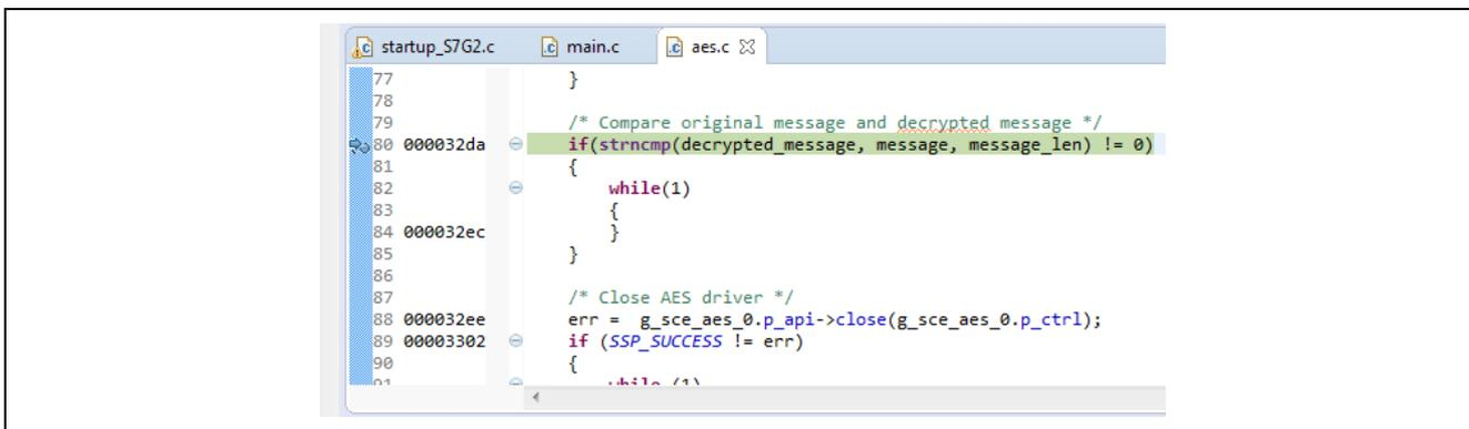
Figure 9 Breakpoint placed at string compare in “aes.c” file
