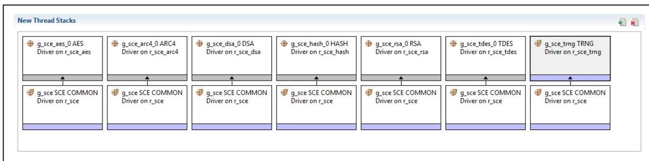
Figure 2 SCE HAL Module Stack (AES, ARC, DSA, HASH, RSA, TDES, and TRNG included)
