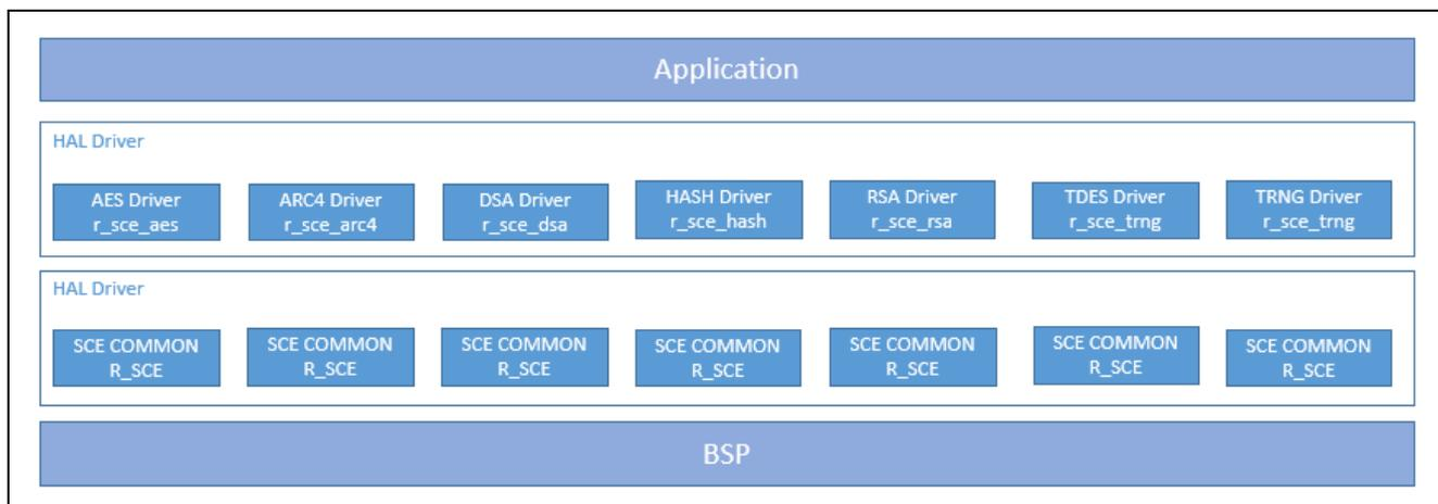
Figure 1 SCE HAL Module Block Diagram
