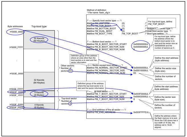
Figure 10.7 Customizing the Boot Type of Flash Memory to Top-Boot Type
