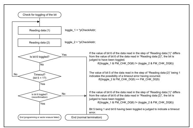
Figure 7.6 Checking for Toggling of the Bit
