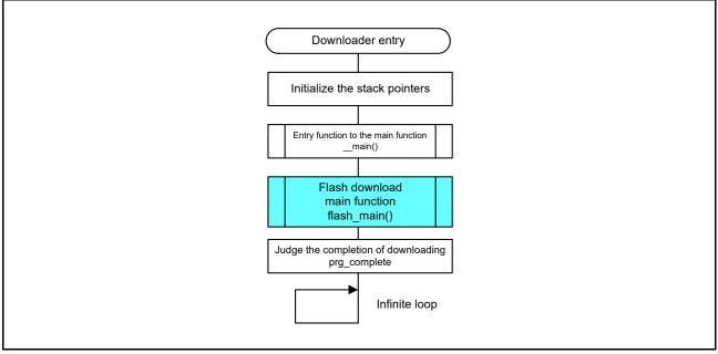
Figure 8.2 Flash Downloader Processing Flow (1/3)
