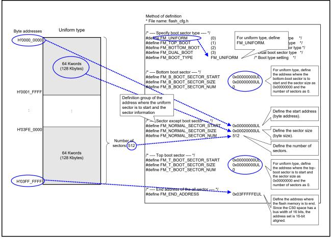
Figure 10.5 Customizing the Sector Size and Number of Sectors of the Uniform Type Flash Memory
