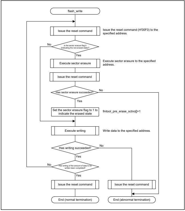
Figure 7.2 Write Interface Function
