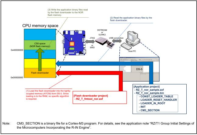
Figure 5.1 Schematic View of Flash Downloader Operation
