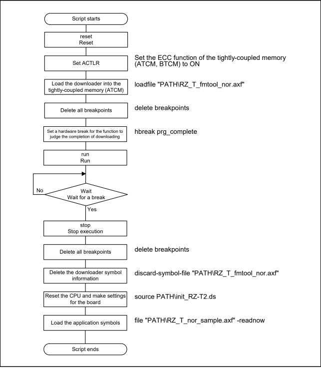
Figure 9.2 Details of Processing by the Application Downloading Script
