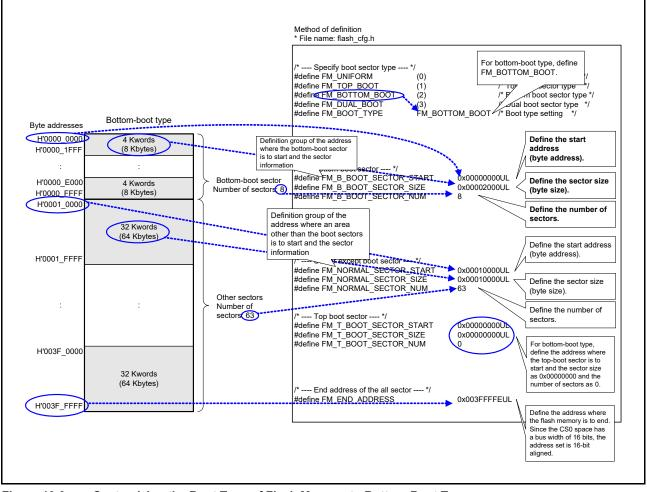
Figure 10.6 Customizing the Boot Type of Flash Memory to Bottom-Boot Type
