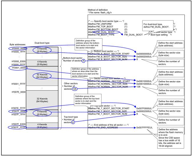
Figure 10.8 Customizing the Boot Type of Flash Memory to Dual-Boot Type
