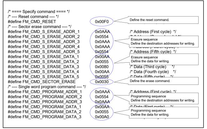
Figure 10.9 Command Definitions of Flash Memory (flash\_cfg.h)
