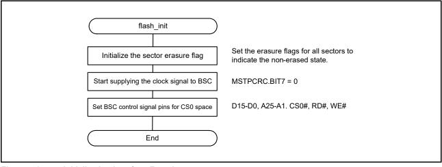
Figure 7.1 Initialization Interface Function
