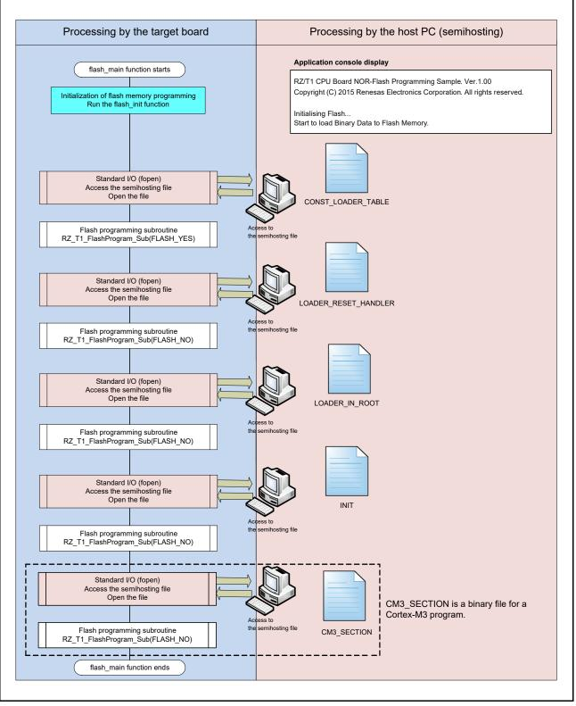
Figure 8.3 Flash Downloader Processing Flow (2/3)
