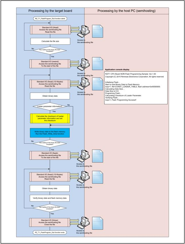
Figure 8.4 Flash Downloader Processing Flow (3/3)
