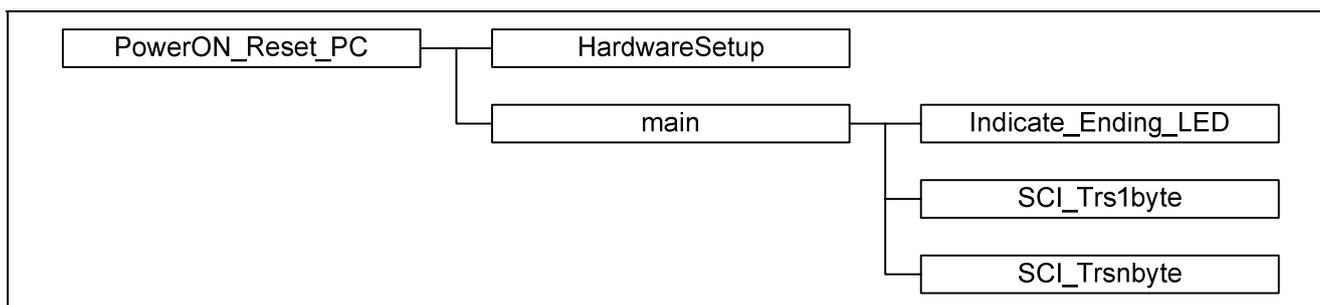
**Figure 11 Hierarchy of Master Device Functions**
