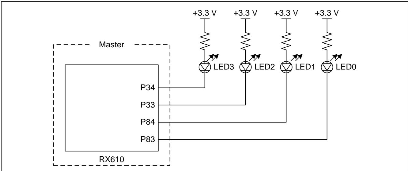
**Figure 9 Master Device LED Connection Diagram**
