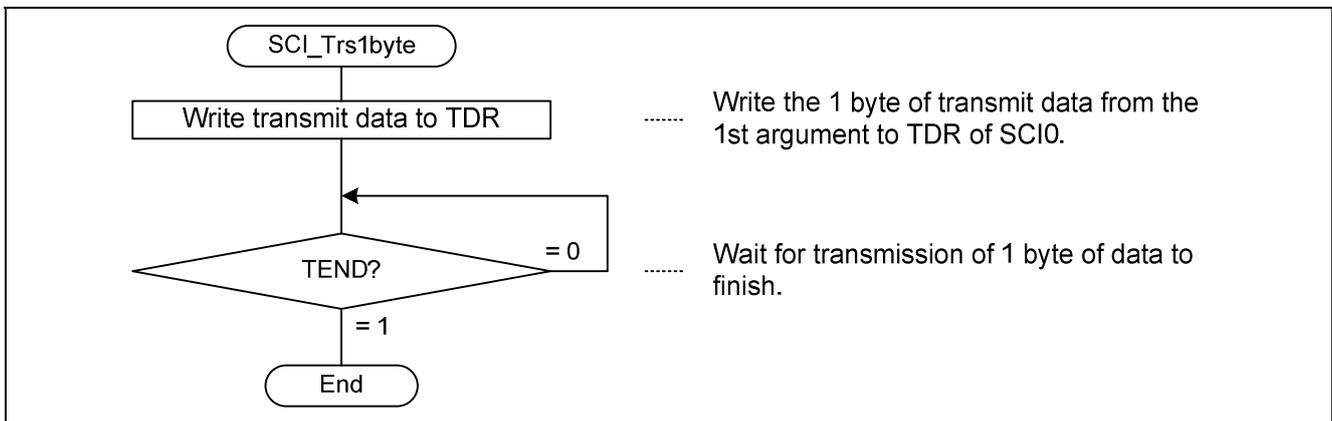
**Figure 17 Flowchart (SCI\_Trns1byte) (Master)**
