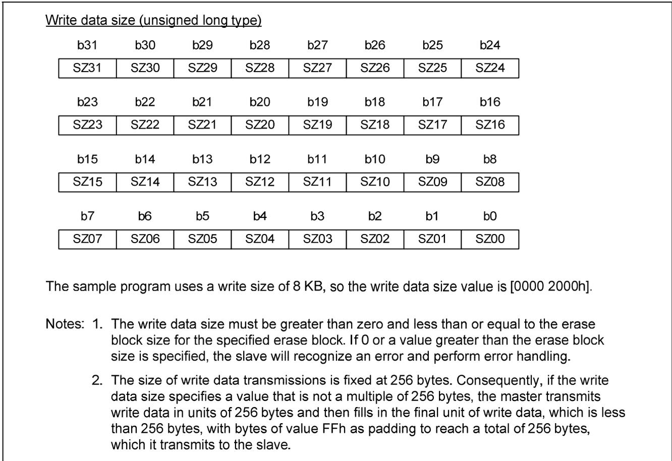
**Figure 8   Write Data Size Specifications**
