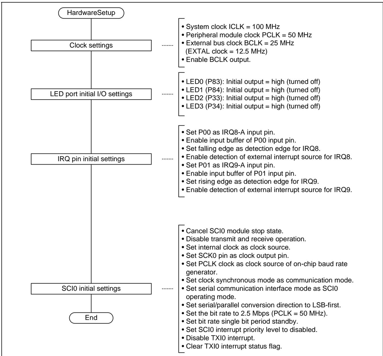
**Figure 13 Flowchart (HardwareSetup) (Master)**
